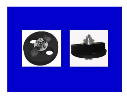
It looks something like this, there is a big rotor, on one side there will be of like elutriator rotor we have described, so the continuous flow rotor is also having applications in different areas of different separations. So, what we have discussed in zonal rotors is, two types of rotors that is, batch type of rotors and we have discussed about the continuous flow rotors. Let us move on, so this was about all different types of rotors, as we have discussed in previous lecture and this lecture.
