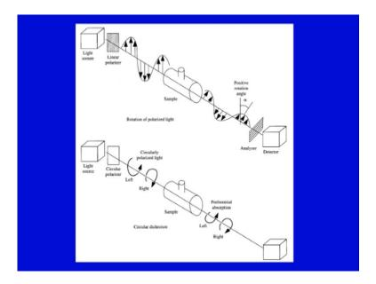
In very simple terms if it is ORD, if you see here on your screen if it you are working with plane polarized light, then what you have is a light source linear polarizer. There is a linearly polarized or plane polarized light, which passes through the sample depending on the sample there will be positive rotation angle or differently it will react and finally, it will be detected after passing through analyzer.
