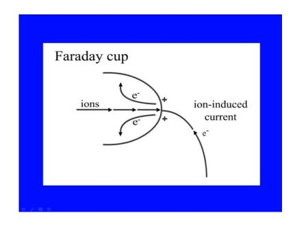
So, a faraday cup could be utilized here, and where secondary electrons are generated.
