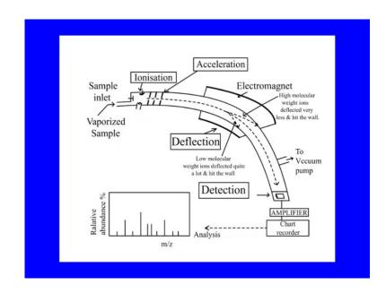
So, if you see here very simple this is a sample inlet here, and this there is a ionization source on ionization, this will be like passing through a particular mass analyzer.
