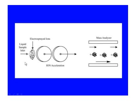
That this is liquid sample these are electrosprayed ions and these are ion acceleration occurs and then finally, the mass analyzer analyzes the sample.
