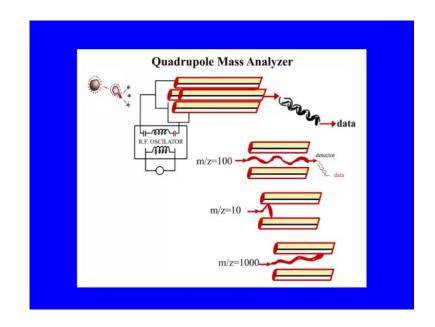
This is typical quadrupole mass analyzer, where you have a RF oscillator there is a mass analyzer, and you get data at different at different frequencies you will get different m to z ratio detected.
