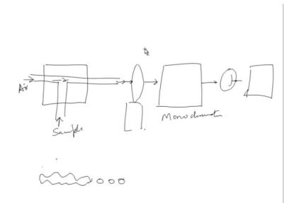
So, what you have is like as we said you have nebulizer, so you have compressed air or oxidant which comes from in this it is a compressed air or mixture with oxidant comes in here. And your sample is placed in here and, so when very high jet of air is passed through then the sample will oscillate and will be attracted or drawn towards this, and it will come in the form of droplets you can just to show you if it is a something like that, it will oscillate in this form.
