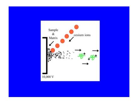
So, if you see here this is schematic of how this ionization occurs in fast atom bombardment, where you have a continuous ions and which bombards and then ions are sample is dissolved from here.
