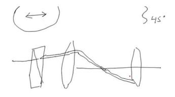
Now, if we go further, if I would like to show this on in a different way it could be like supposing there is a prism here and there is a condenser lens which will be focusing the light. Than the light comes in here and then light is divided into two and the adjacent light goes in here, which will enter the condenser and then will be focused onto the specimen plane.
