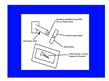
Now, this figure shows in here a microtome. So, microtome has this. This is a microtome arm. This microtome arm, if you can see here is specimen, which is embedded specimen paraffin or wax, which is hardened is put in here. This microtome arm is moved up and down rapidly. It moves through this glass blade or metal blade. There is a trough, water trough here where the sections fall. These are sections. Like I said, there would be around, what you call 1 to 10 micrometer sections here.
