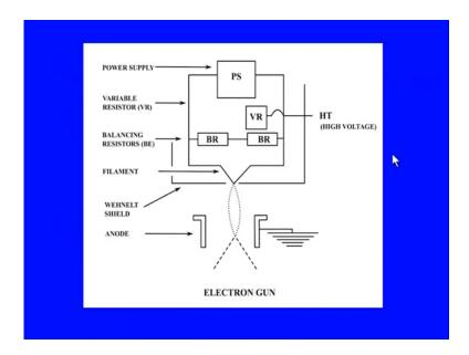
Now, let us see how this looks likes. This is an electron gun or emission source. Here if we see this figure there are lot of different electrical things power supply variable resistors balancing resistors. What we are interested in are the, cathode and anode. The cathode is this simple V shaped tungsten filament. This is when heating gives you electrons.
