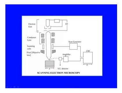
Now, let us see the optics. We have discussed this; let us try to understand through this figure. Like I said earlier, we have shown you electron gun but only difference is that it is 2 to 30 kilovolt anode. It is at a negative potential than anode. There is a difference here from transmission electron microscope. If you can see here rather than having a specimen at somewhere between the specimen is placed at the end of the column.
