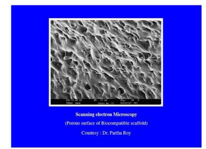
This is a scanning electron microscope picture. Here, is of a porous surface of biocompatible scaffold. All pictures have been provided by Doctor Partha Roy. They have been taken in his lab. Thanks to him. Here, we complete our section on the microscopy. I hope you have understood the basic concepts and details of different microscopy techniques. We have discussed in here, we have gone through light microscopy techniques.
