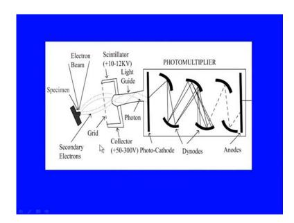
A specimen is here, little tilted electron beam is coming from the top. It is scanning, now this is a coated surface. It becomes conductive surface. The secondary electrons generated here, will be focussed or collected by a collector. This is a positive potential of around 50 to 300 volts. This collector attracts the electron and then they are passed into the scintillator. This is at positive potential of 10 to 12 kilovolt. These scintillators convert them into photons.
