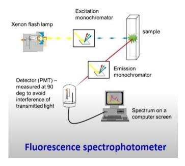
In the fluorescence spectrophotometer, we have a light source, which is the xenon flash lamp. It provides the energy needed to excite the sample. Following that, we have the excitation monochromator. It selects the exact wavelength of light used to excite the sample. Then we have the sample holder.
