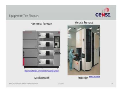
There are several vendors to will sell you a high-quality oxidation furnace. Older technology or small wafer models tend to be the horizontal reactor. Production tools and large area wafers tend to have a vertical tube. The reason for vertical versus horizontal is purely for a space constraint. The cleanroom is a very expensive real estate, so, you do not want very large equipment and one way to save space is to have a long tube lying vertically instead horizontally as it takes less space.
