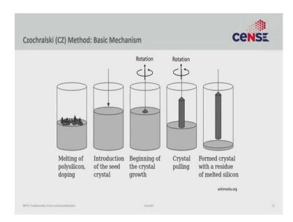
The basic mechanism of the Czochralski method is given in this slide. You start by melting the polysilicon feedstock. Heat it above the melting temperature of silicon, and once it has completely melted you can add a certain amount of dopants. The number of dopants you add will define the resistivity of the eventual wafer. Because you are dissolving it in a homogeneous solution the doping that you would get in this melt would be hopefully uniform.
