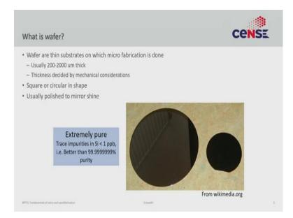
So, what is a wafer? As the name suggests wafer is a thin substrate on which the micro and nanofabrication is done. The name comes from historical reasons Here is an example of a silicon substrate and you can see that it looks like a thin slice or wafer and that is why the word wafer.
