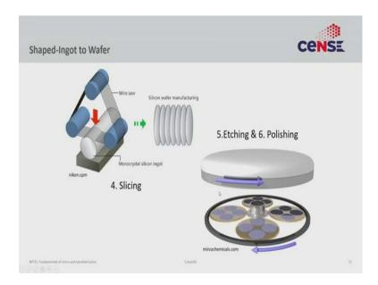
This process is similar to how a log is converted into round shapes. The diamond wire saw is used to cut the ingot down into thin slices. The distance between the wire saw decides the thickness of the wafer. This sort of sawing leaves certain striations on these wafers which are called saw marks. In order to get a smooth or mirror shine, you need to polish these substrates. That is done in this etching and polishing set up.
