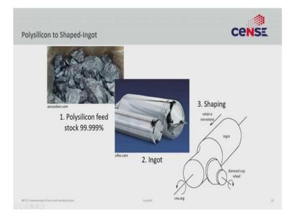
We start with polysilicon, which is silicon that has been purified to 99.999 %. For most material or chemical applications, it is essentially pure. So, that is the purest silicon you can buy and comes in chunks. What you then need to do is convert this polycrystalline, extremely pure, but not pure enough silicon into a silicon wafer. The first step is creating a single crystalline ingot.
