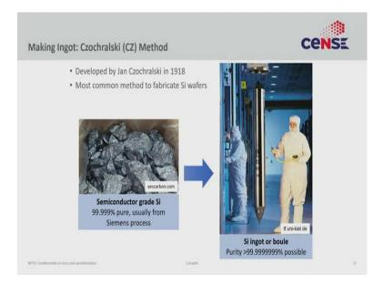
Let us go into the detail of each of these steps. First is making the ingot from the polysilicon feedstock. The polysilicon feedstock is generally 99.999 % pure, and it comes from Siemens process that you can read up on the internet if you are interested.
