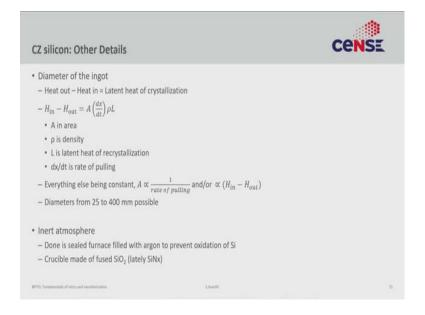
Another very important detail is the diameter of the ingot. As silicon technology has matured we have started growing larger and larger ingots. So, how do we control that process? we simply look at the thermodynamics. Assuming this is a closed system where we are putting in some amount of heat by heating the crucible, some amount of heat is being lost and the rest must be taken by the latent heat of crystallization, which is described by this expression.
