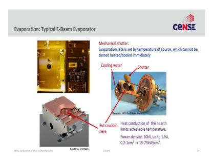
E - Beam evaporators are a little more complicated as they have water-cooled hearth inside the vacuum chamber. It is often made of copper to make it thermally conductive.
