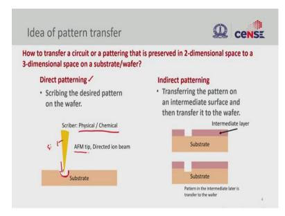
After understanding the importance of pattern transfer, let us examine how to direct patterning and indirect patterns are made. We will see how do we transfer a 2-dimensional structure into 3-dimensional features onto the wafer.
