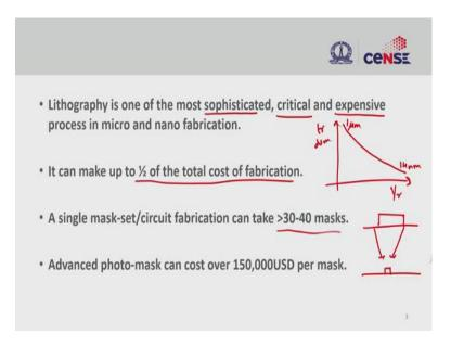
Lithography is one of the most sophisticated processes. We saw a decrease in the transistor dimension over the years if we look at the CMOS technology evolution. So, we started from 1  $\mu$ m technology, and now we are at less than 14 nm node. So, the whole evolution of reduction of the size of the transistor is primarily driven by lithography.
