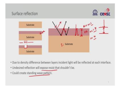
The above image shows substrate and coated with photoresists. When we illuminate the resist with light using a mask, a trench is formed on the exposed region if the resist is positive. The process can be contact or proximity, or projection lithography.
