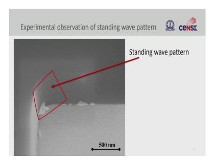
The scanning electron microscope image shows the wavy pattern on the sidewall of the photoresist after development because of the absence of an anti-reflective coating. This non-uniformity on the photoresist will be transferred to the underlying silicon during dry etching.
