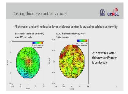
The above slide shows thickness variation of photoresist over 200mm wafer on the left and thickness variation of BARC over 200 mm wafer on the right. The range of thickness variation of photoresist is about 5 nm, while for BARC, it is about 1 nm. This is achievable with the current technology.
