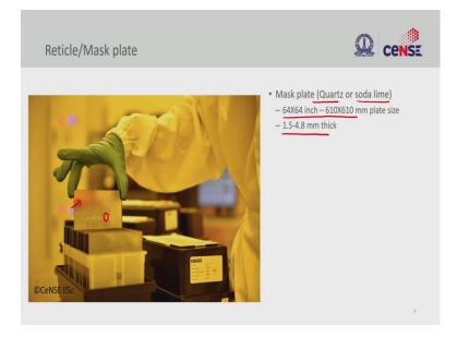
The image shows a mask plate from Nano-Science Department at IISC. The mask plate shown has chrome as opaque regions and openings that are transparent for the light to go through. The mask plate can be either quartz or soda-lime; both are transparent in the region of interest. And the mask plate size can vary based on the tools and the circuit to define. The thickness of the substrate also can vary; e.g., a larger mask uses thicker plates for mechanical strength.
