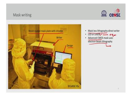
The above picture shows an engineer holding a resist coated mask with chrome and the monitor with design, which is fed to the writing machine. When the mask is loaded into the tool, it will start writing the layer onto the photoresist. For the mask, the writing process is used, and the tool is shown in the above slide.
