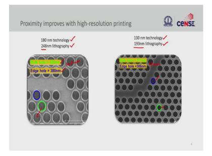
And, this is an example of how to improve your resolution. And, proximity effect is a classic example of resolution enhancement. On the left side, you see 180 nm technology and 248 nm illuminating optics. Say, we are illuminating the same object and the bulk holes. As a result, the holes that are inside got a hole diameter of 420 nm and the edge holes got only 380 nm. This is a classic proximity effect, the edge effects.
