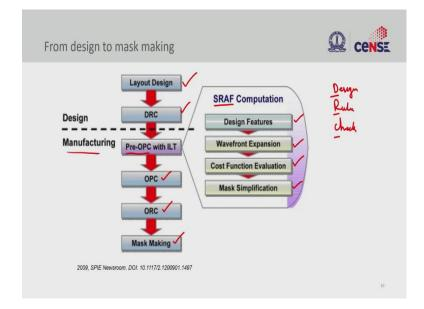
And, this is a process flow to reproduce that mask. So, you start with a layout that is coming from your design and then you do Design Rule Check (DRC). DRC is to check if all the design rules are followed or not. For instance, if the lithography limit is only 50 nm and then in your layout/circuit, if you are asking for 50 nm it is a violation because it cannot be reproduced.
