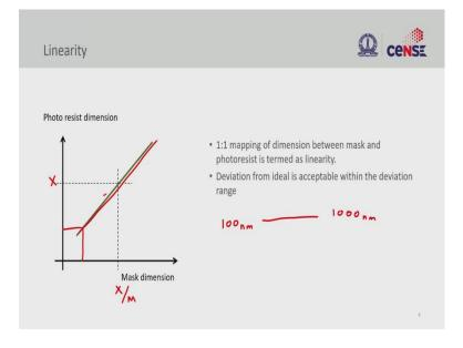
And, the next thing is the linearity. So, what is linearity? So, we want to have one to one mapping of the dimension between mask and photoresis. So, if the mask dimension is you know some 'x'. Of course, this is taking into account the magnification factor and on the mask as well the wafer you want to have the same dimension. So, this is what we call linearity.
