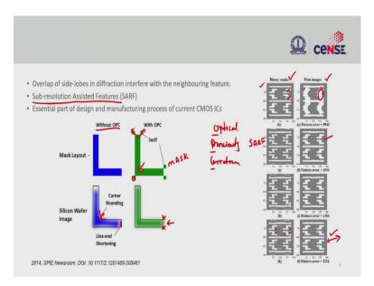
And, the other thing to circumvent the proximity issue is by using assist features. So, we saw this L shape earlier with some rounded corner. So, this is a simulation image on the left side without OPC (Optical Proximity Correction). So, if you do not do any optical proximity correction you get two things; one is line-end shortening, the other thing is the corner rounding.
