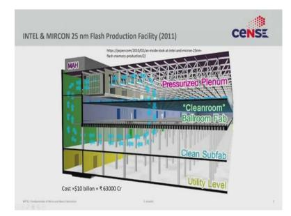
So, let us start with an example. This is a fab that was jointly made by Intel and Micron, which are two very large semiconductor industries and they set up a joint facility in Utah, sometimes in 2011 for 25 nm node. The rest of the details do not matter but concentrate on this figure that they released describing what the architecture of their cleanroom looks like.
