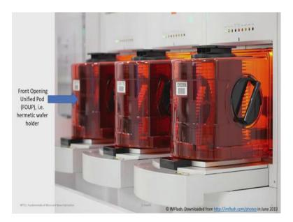
Over each tool, these orange-colored boxes store the wafers. Wafers are typically processed in batches of 25 or 50 and each of these boxes stores the wafer. The boxes are completely sealed. Despite this being a clean room, the wafer never sees this clean room but a much purer environment inside this pod. Removal and addition of the wafers into the pod and outside the pod is all managed by robots. These are called foups or front opening unified pod.
