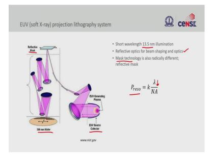
So, the continuation to optical lithography in terms of resolution is extreme UV lithography. So, this extreme UV lithography is being considered as the next step towards addressing the resolution needs by reducing the wavelength. So, here we are looking at 13.5 nm illumination wavelength. So, this is a soft X-ray type. So, the rays are generated from a plasma source, and then used in reflective optics which is very different from the transmission optics that we have seen in optical lithography.
