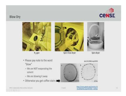
Once you are done with rinsing there is typically a step of blowing dry the wafer. Please note the word 'blow'. The idea is not to dry the liquid on top but to push it off the wafer on to some absorbent cloth. You do not want to dry the water because when you dry the water on a surface you tend to form stains. This is what I call coffee rings. Coffee that dries on top of a table will leave a stain as the solvent evaporates away, the solute just precipitates out on top of the surface.
