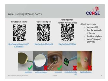
A few other wafers do's and don'ts that you may look at in these videos. To summarize it all, always use personal protective equipment, hold the wafers from the edges, never hold the wafer with hand and always blow dry. Make sure that the tweezer doesn't touch the device; hold the small substrates from the edges. Any die once touch by hand will always have sodium-potassium contamination which is not good for the device.
