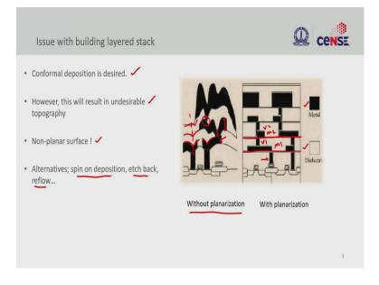
Let us look at some general expectations from the wafer fabrication process and the issues we face when building a multi-layer stack. So, we tend to use conformal deposition, which gives a very good fill but results typically in topography on the surface; that means it will not be flat anymore, so we call non-planar surface.
