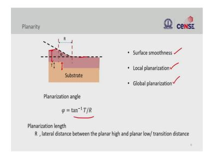
Here is how we characterize the planarity. Planarity is nothing but the angle between the global flatness or the local flatness that we have. It strongly depends on the topography that we start with and the material we have, and the flatness we are looking for.
