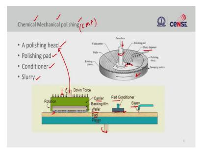
So we use chemical mechanical polishing. As the name suggests, we use chemicals and mechanical force to do polishing. The setup has these four critical elements; a polishing head where the wafer is loaded, a polishing pad, a conditioner, and a slurry.
