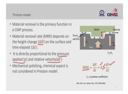
So, let us look at the mechanism used in removing the material. We shall see how the pad, the slurry, and the pressure between the wafer and the pad affect the material removal.
