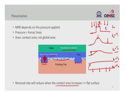
This is how the pressure distribution will look like. On the top is the wafer and the bottom is the polishing pad. This red dot is showing the pressure distribution. When the wafer is flat, we do not have much pressure that is being applied. So, there is no removal at all because it is a physical process; we are pressing against the surface and rubbing it.
