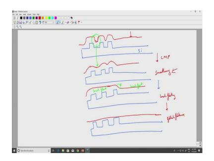
Let us look at the working of a CMP process. So, let us start with a very simple structure. We have a silicon substrate with a certain topography, and we deposit a material, let us say, silicon dioxide, on the top of it. Now the silicon dioxide is going to follow the topography. The goal is to flatten the topography and level the surface.
