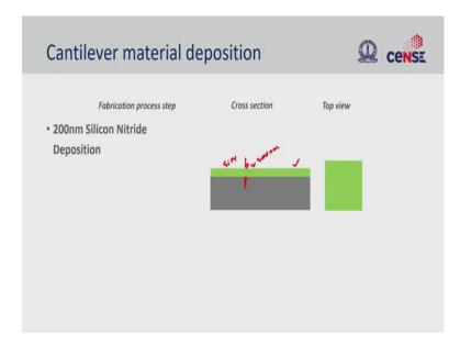
The next process is cantilever material deposition. As mentioned earlier, we are using silicon nitride as the cantilever material of approximately 200 nanometres. The above slide shows the cross-section image of 200 nm silicon nitride on the silicon substrate, and the top view shows the uniform film as it is a blanket deposition. We are going to use low-pressure chemical wafer deposition, a high-temperature furnace process for silicon nitride deposition.
