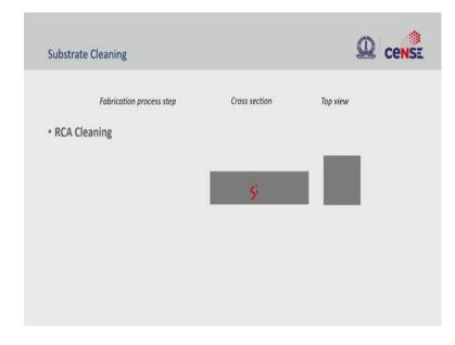
The first step in fabrication is substrate cleaning. Here we use a wet process, RCA, to clean the silicon wafer to remove any contamination on the surface.
