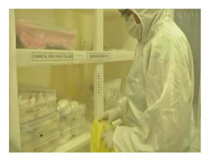
To carry out the wet process is to wear personal protective gear, protection from any chemical safety hazard. It includes safety sleeves to avoid any acid spill or splashes will fall on hands, then the apron to prevent any acid or any chemical spill onto the body. And the next is to protect the face and head using a face mask. Once completely dressed, we enter the wet bench, consisting of multiple benches for various wet processes.
