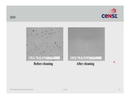
SEM is another common example. Here, you see some particles on the surface that are removed after cleaning. This works as long as the particles on the surface are not very sparse but have a reasonable amount of density.
