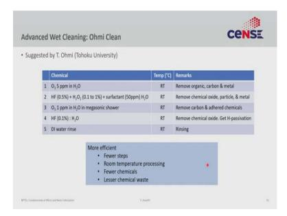
This is what you have to do before the critical steps. The industry has moved towards more efficient cleaning processes that require fewer steps, not as complicated as what we discussed in the last slide. A room-temperature process is important to save time and cost and fewer chemicals because when you are doing this for very large batches, for a long time, the cost adds up because these are extremely pure chemicals and very expensive.
