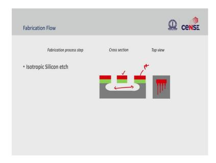
To release silicon nitride cantilever, the underlying silicon is etched isotropically using ICP RIE tool. Here SF6 gas is used for isotropic etch silicon.
