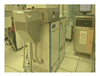
We use the ICP RIE reactor for anisotropic silicon nitride etch and isotropic etch of silicon and then remove the photoresist. The tool consists of an inductively coupled plasma (ICP) reactor that generates high-density plasma, and the wafer is going to sit at the bottom.
