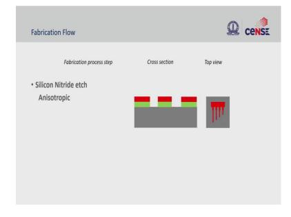
To transfer the pattern from photo resist to the film, silicon nitride is anisotropcally etched using ICP RIE tool.
