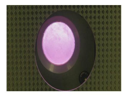
When the required pressure and gas combination for silicon nitride is achieved, the plasma will strike, as shown in the above image. Plasma is generated when the excited gas molecules come to the ground state, emitting a photon. Plasma goes off when the etching is done.
