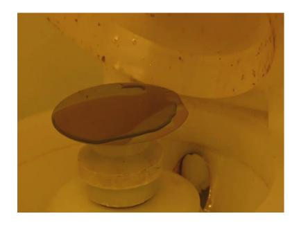
The wafer is placed on the spinner and an appropriate program for rotation is selected. A sufficient amount of photoresist drop casted on the wafer.
