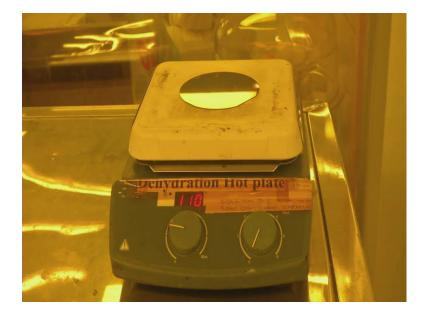
Dehydration bake is done at around 110 degree C, slightly above the boiling point of water, so that all the water present in the wafer is evaporated. After dehydration, the wafer is taken for coating photoresist using spin coating technique.
