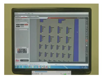
Microscope image shows silicon nitride of various shapes and sizes cantilevers on a silicon substrate. The cantilever view is then zoomed in to check the quality of the cantilever fabricated.
