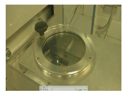
The wafer that needs to be etched is loaded in the load lock, and it is pumped. Once the required pressure is reached, the robot arm will transfer the wafer into the chamber.
