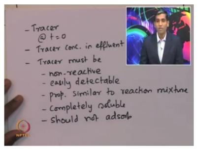
So, the method to do that is basically to inject a tracer. We need to inject a tracer into the reactor. And let us say, at time t = 0, a certain concentration of tracer is actually inserted, injected into the reactor. And then, the effluent concentration the tracer concentration in the effluent is measured. So now, if we measure the tracer concentration in the effluent, then this gives an idea about the non-ideal behaviour of the reactor.
