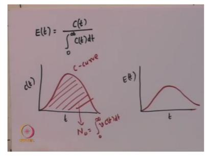
So, from here, we can easily see that the residence time distribution function E t is essentially given by the concentration of the tracer at any time divided by the total amount of tracer that is actually leaving the reactor. Or the total amount of tracer that is actually entering the reactor. So, if I plot this function. So, suppose the concentration versus time graph. So, the effluent concentration as a function of time, if it looks like, suppose if it is a bell-shaped curve.
