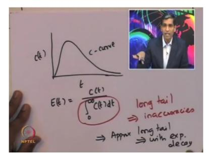
If I look at the concentration curve, in certain situations there can be a very long tail which is present in the c-curve. So, this is the c-curve. So now, the concentration curve has to be integrated. Remember that E of t is basically given by c t divided by integral 0 to infinity C t d t provided that the effluent volumetric flow rate is constant, there is no dispersion, etcetera. So, in order to perform such an integration, one needs to do a numerical integration of this curve, this c-curve.
