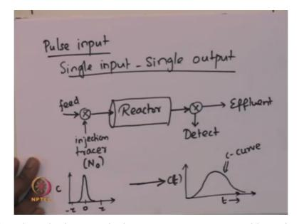
So, let us look at the pulse input method. So now, suppose we consider a single input-single output system. That is, suppose if there is a reactor. And then, there is a single input stream to the reactor and single output stream to the, from the reactor. And suppose if there is a feed stream which is present here. And let us say that we put a an inject, we inject the tracer along with the feed which actually goes into the reactor.
