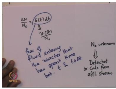
That is = E of t into d t. So, what is this E of t represent? E of t is the RTD function which is v into C t divided by N nought. What it represents is, it basically describes how much time different fluids elements are actually spent in the reactor. So, this quantity E of t which is the residence time distribution function, it quantifies or describes how much time different fluid elements have actually spent or have resided inside the reactor before they leave the reactor.
