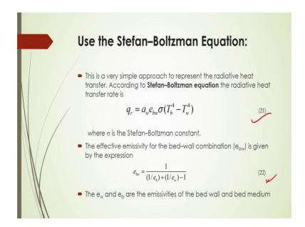
Now, if we consider that Stefan Boltzman equation very simple approach to represent to the radiative heat transfer, in this case, according to that Stefan Boltzman equation, the heat transfer rate can be estimated by this equation number 21; whereas, sigma is the Stefan Boltzman constant the effective emissivity of the bed wall combination is given by expression equation 22, here in this case, e w and e b are the emissivities of the bed wall and the bed medium.
