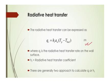
And this radiative heat transfer can be expressed by this equation number 20, this is the standard equation to represent and where q r is the radiative heat transfer rate on the wall
