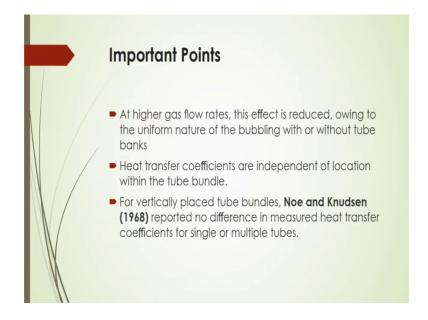
We will see the effect is reduced that will owing to the uniform nature of the bubbling with or without tube banks heat transfer coefficients are independent of location with the tube bundle for vertically placed tube bundles, Noe and Knudsen, 1968; reported that there will be no difference in the measured heat transfer coefficients for the single or multiple tubes.
