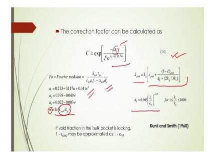
This is a function of that is Fourier modulus which is defined as by this equation here and this one important parameters like a 1, a 2 and a 3; this a 1, a 2, a 3 are a function of ah; that means, for void fraction of the solids they are in the bed and this w this w is a defined as l n k p a b by k g; this is actually the logarithm of the ratio of this; what is that that is thermal conductivity of the packet particles to the what is that gaseous.
