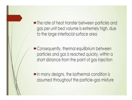
Now, the rate of this heat transfer between the particle and gas per unit bed volume is extremely high. So, due to the large interfacial surface area, if we decrease the if we decrease the size of the particles, you will see that more surface area of the particles will be inside the bed and because of which you will get the more surface area for the transferring of heat from this sub particle to the medium.
