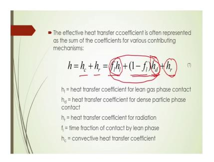
Now, the effective heat transfer coefficient is often represented as the sum of the coefficients for various contributing mechanisms like h will be is equal to h c plus h r; what is h c? H c is called convective heat transfer coefficient and h r; h r is called the heat transfer coefficient for radiation. Now, this can be denoted by this h c is nothing, but f l into h l plus 1 minus f l into h d plus h r here.
