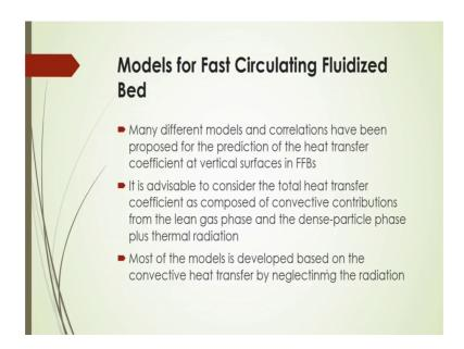
Now, many different models and correlations have been proposed for the prediction of the heat transfer coefficient at vertical surfaces in first circulating fluidized bed condition it is advisable to consider the total heat transfer coefficient as composed or convective contributions from the lean gas phase and a dense particle phase plus thermal radiation most of the models is developed based on the convective heat transfer by neglecting the radiation.
