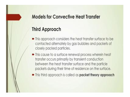
And the third approach the third approach to represents this convective heat transfer that considers the heat transfer surface that is to be contacted alternately by gas bubbles and packets of closely packed particles.
