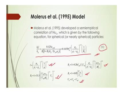
So, in this case; based on this consideration of this gas and particle movement, Molerus et al 1995; they have developed one semi empirical correlations for this Nusselt number of this convective heat transfer coefficient, in this case, they have given this equation for spherical or nearly spherical particles by equation number 11.
