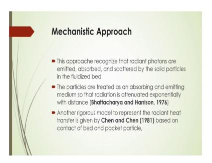
Whereas, in this mechanistic approach; that recognize that the radiant photons will be emitted and will be absorbed and will be scattered by the solid particles in the fluidized bed the particles that are treated as an absorbing or emitting medium. So, that the radiation is attenuated exponentially with the distance another rigorous model that is developed to represent to the radiant heat transfer given by Chen and Chen, 1981; which is based on the contact of bed and packet particles.
