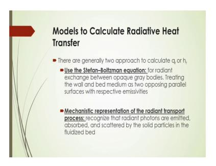
Models to calculate radiative heat transfer there are generally 2 approach to calculate this q r or h r use the Stefan Boltzman equation and mechanistic representation of the radiant transport processes the Stefan Boltzman equation, in that case, radiant exchange between opaque gray bodies will be considered and treating the wall and bed medium as 2 opposing parallel surfaces with the respective emissivities that is actually considered to express the radiant heat transfer rate.
