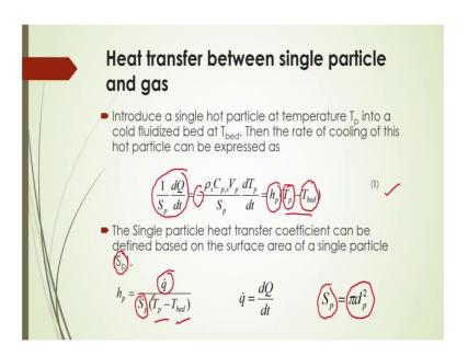
Now, anyway what should be the then heat transfer between single particle and gas because we have to know the basic fundamental law of the heat transfer from one phase to another phase, if we consider one single particle, then how heat will be transferred from this single particle to the gas there.
