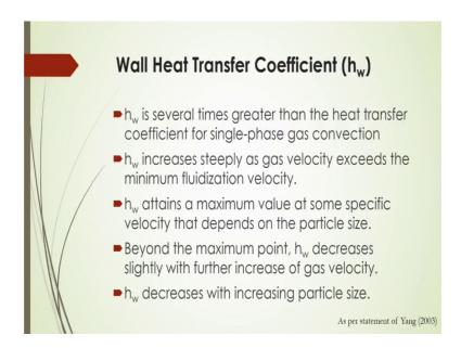
And this wall heat transfer coefficient; of course, there will be a change because of different operating conditions and it is seen that that wall heat transfer coefficient will be several times greater than the heat transfer coefficient for single phase gas convection and this wall heat transfer coefficient increases very steeply as gas velocity exceeds to the minimum fluidization velocity.
