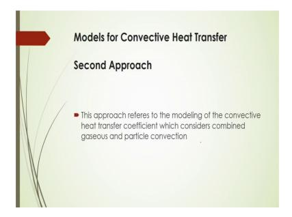
Second approach is that who is refers to the modeling of the convective heat transfer coefficient which considers the combined gaseous and particle convection there.
