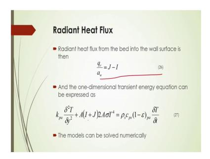
Whereas in this equation A and S are the volumetric absorption coefficient and volume volumetric scattering coefficient respectively the radiant heat flux from the bed into the wall surface is then calculated by this equation number 26. Once you know that this forward and backward radiant fluxes and one dimensional transient energy, equation can be expressed by the equation number 26 with respect to that what is that this backward and forward radiant heat fluxes.
