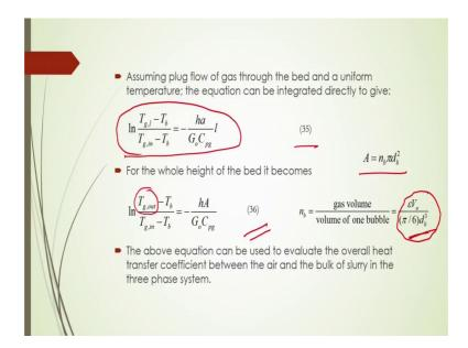
Now, assuming plug flows of the gas through the bed and uniform temperature the equation can be then integrated directly to give this equation number 35 from which you will be able to calculate what should be the temperature at a certain length of the three phase fluidized bed, once you know this equation and for the whole bed what should be the heat transfer coefficient and what should be the temperature profile, you will be able to calculate from this equation number 36.
