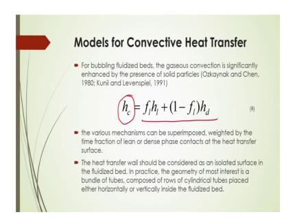
Now, what are the different models by which you can express this or analyze this heat transfer coefficients, let us consider fast that convective heat transfer coefficient for bubbling fluidized bed, the gaseous convection is the significantly actually enhanced by the presence of solid particles and because of which there will be a enhancement of the heat transfer are in this bubbling fluidized bed phenomena.
