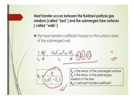
Now, heat transfer occurs between the fluidized particle or gas medium; that is called bed and the submerged bed surfaces that is called walls the heat transfer coefficient based on the surface area of the submerged wall; that will be represented by this equation number 6 here. So, in this case submerged wall, then heat transfer coefficient will be represented by this h w that is called Heat transfer coefficient wall heat transfer coefficient here.
