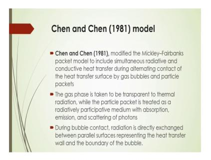
And scattering of photons during bubble contact the radiation is directly exchanged between parallel surfaces representing the radiant heat transfer wall and boundary of the bubble.
