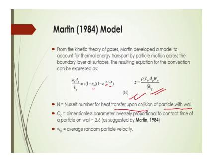
Martin, 1984; they have developed this equation to actually calculate the convective heat transfer coefficient in the dense bed medium based on the kinetic theory of gases and martin developed the model to account for thermal energy transport by particle motion across the boundary layer at surface and they have developed this equation number 16 to calculate the heat transfer coefficient.
