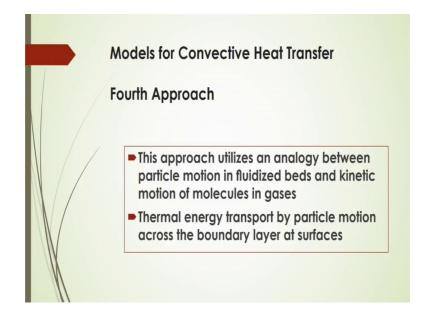
Now, as a fourth approach you can calculate the convective heat transfer coefficient, in this case utilizes an analogy between particle motion in fluidized beds and kinetic motion of the molecules. Molecules in gaseous and also thermal energy transport by particle motion across the boundary layer at surfaces.
