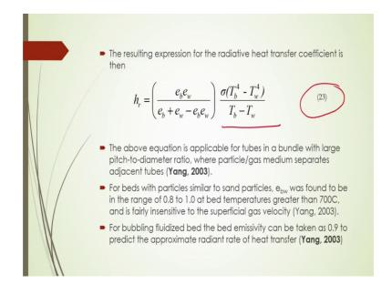
The resulting expression for the radiative heat transfer coefficient is then h r that will be is equal to e b e w by e b plus e b e w minus e b e w into this fraction that is given in equation number 23; the above equation is applicable for the tubes in a bundle with large speeds to diameter ratio whereas, particle or gas medium separates that is adjacent tubes there.
