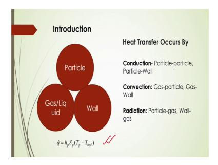
And it is well known that there are 3 types of heat transfer mechanism are there; one is conduction, another is convection and other one is called radiation. So, both 3 mechanism may happen in the fluidized bed during this heat transfer operation.
