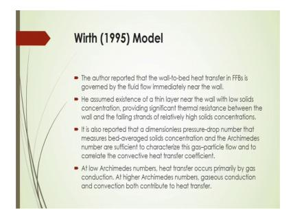
There is one important model that is called Wirth, 1995 model; this model that according to their model author reported that the wall to bed heat transfer in the first fluidized bed is governed by the fluid flow immediately near the wall he assumed existence of a thin layer near the wall with low solids concentration providing significant thermal resistance between the wall and the falling strands of relatively high solids concentrations.
