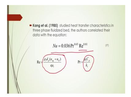
As per Kang from the experimental data, the equation 37 can be represented to predict the heat transfer coefficient in the three phase fluidized bed where this is again is a function of Prandtl number and Reynolds number, here Reynolds number will be defined as by the fluid mixture properties and the Prandtl number also, it is a mixture of the liquid here.
