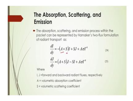
Now, how to actually estimate this absorption scattering and the emission the absorption scattering and emission process within the packets can be represented by the Hamaker's two flux formulation of radiant transport which can be given by this equation 24 and 25 for the forward and backward radiant fluxes and this forward and backward radiant fluxes is represented by this or denoted by this I and J.
