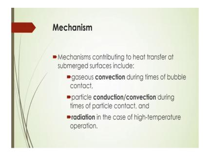
Now, what are the different mechanism of this heat transfer at the submerged surface that will include to the includes the gaseous convection during times of bubble contact and the particle conduction or convection during times of particle contact and radiation in case of high temperature operation.
