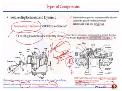
When we come to the type of compressor there are variety of the compressor available in the market and those can also be designed to meet the specific need broad classification is positive displacement is dynamic compressor within this classification the reciprocating compressor and centrifugal compressor are widely used in the natural gas industry and primarily it is reciprocating compressor that is having more application in the natural gas industry.
