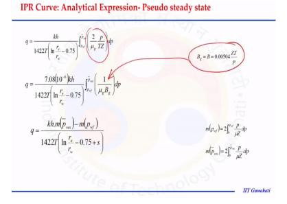
Like here it is shown the formation factor can be used to substitute some of the values here it can be substituted here in this form and we can get the expression for q versus pressure draw down and this relationship is called IPR
