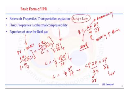
And that can be done considering how reservoir properties are going to contribute for the transportation equation that can be represented by the Darcy law. Darcy law simply says for the radial flow condition q = Ak / Mu del p / del rho k is a permeability of formation which is along the fluid to travel from one point to another point or from reservoir domain to well bore.
