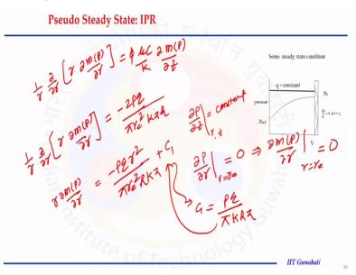
Now what happens under the pseudo steady state condition if we see by the definition of pseudo steady state we are having this boundary condition or the condition will says the pressure change with respect to time is constant. So the basic IPR equation on the right hand side what we are going to get is a constant value instead of 0 that we got in steady state condition pseudo steady state condition we are going to get this relationship which is the function of
