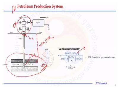
In flow performance relationship related this segment of our conventional petroleum production system. If we look the overall picture of production system we can divided this in 3 segment this is IPR where the flow is happening from reservoir a complex domain that is pores in the nature gases stored there in the pores region because of the permeability in the reservoir the gas is flowing from reservoir to well bore.
