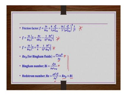
So, then we got this expression. Then using this expression we further calculated the friction factor as well. The friction factor that we have got this one which we have written in terms of the properties of a material that is density, viscosity and then yield stress etcetera, ok. Yield stress is also property of the material; characteristic property of the material like density etcetera that we have for other properties like.
