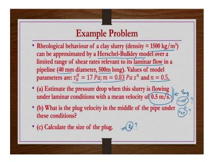
So, one material density is having 1500 kg per meter cube is flowing through a pipe under laminar flow conditions pipe dia is 40 mm, length is 500 meters ok. The material can be represented by Herschel-Bulkley fluid model where  $\tau_0^H$  is 17 pascal, m = 0.83 and n = 0.5 right.
