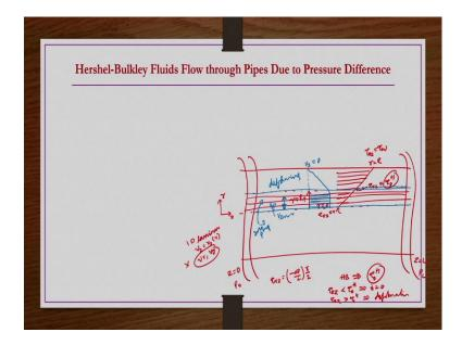
So now, that is what we are going to see now. Herschel-Bulkley fluids flow through pipes due to pressure difference right. So, now let us say this is the pipe that we have and then this is the centre of the pipe or circular tube whichever you are taking.
