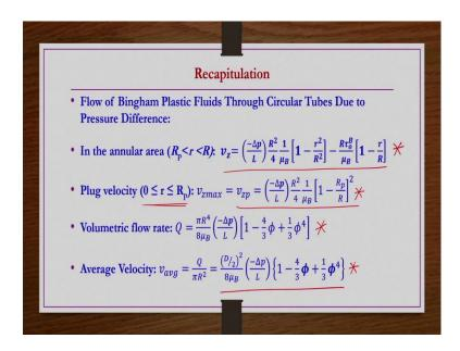
So, flow of Bingham plastic fluids through circular tubes due to pressure difference. Then if you follow the process that we have been doing in order to get the velocity profile etcetera. We get velocity profile for the annular region that is between  $r = R_p$  to R; we get this expression.
