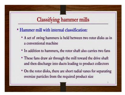
Classifying hammer mills or hammer mills with internal classifications, what we have a set of swing hammers is held between two rotor disks as in a conventional machine but in addition to hammers, the rotor shaft also carries two fans. Why these fans are required? These fans draw air through the mill toward the drive shaft and then discharge into ducts leading to product collectors.
