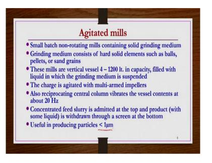
So, now we go to the agitated mills. Agitated mills are a kind of small batch non-rotating mills containing solid grinding medium. Grinding medium in general consists of a balls, solid elements such as balls, pellets or the sand grains. These mills are in general vertical vessels having capacity 4 to 1200 litres filled with a liquid in which the grinding medium is suspended, the liquid has to be non-reactive and non-corrosive.
