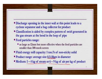
Discharge opening in inner wall at this point leads to a cyclone separator and a bag collector for product as explained. Classification is aided by complex pattern of swirl generated in the gas stream at the bend in the loop of pipe. Feed particles range, it can handle as large as 12 mm particles but it has been found that fluid energy mill works effectively, feed particle size is smaller than 100 mesh screen. However, it can also handle the particles up to 12 mm size large as well.
