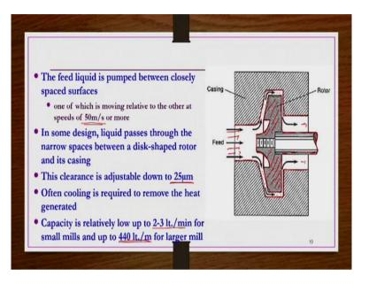
So typical schematic if you see we have a kind of casing like this. Casing that is for a colloid mill like this and there is a rotor, with a kind of you know disc kind of shapes, some different types of disc are possible. These discs are in general connected to a kind of rotor which rotates. It rotates in this direction which are we are we need to rotate. It can be rotated in either of the direction but in general they are rotated in one single direction.
