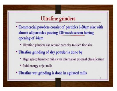
So, let us start with a you know for the case of a ultrafine grinders so in general what happens commercial powders need to have a particles in the range of 1 to 20 microns on the average. Sometimes particles may have a, you know slightly oversized compact the 20 microns but almost all particle should pass through 325 mesh screen having opening of 44 microns in general. So, that is the requirement in any of the commercial powder in general.
