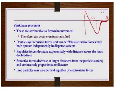
So we see individually, perikinetic processes, these are attributable to the Brownian movement, that is you know even when you have a kind of stationary fluid without any bulk motion, so at the molecular level, the molecular vibrations, interactions, molecular rotations et cetera, those kind of things will be there. Those kind of vibrations, rotations of the molecules induce some kind of motion, that is known as a kind of Brownian movement or the Brownian motion. So
