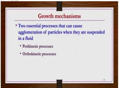
So what are the growth mechanisms? Growth mechanisms, two essential processes that can cause agglomeration of particles when they are suspended in a fluid rather than in a kind of individual solid phase. When you suspend these fine particles in a fluid then two essential processes may take place, they are nothing but perikinetic processes and then orthokinetic processes.
