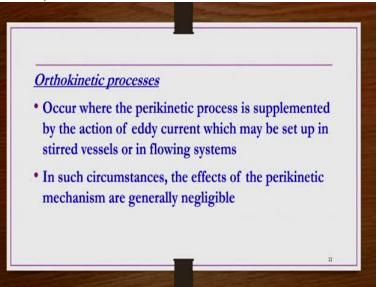
Whereas the orthokinetic processes which are occur where the perikinetic process is supplemented by the action of eddy current which may be set up in stirred vessel or in a flowing system. If the fine particles along with a fluid you may be taking in the kind of vessel and then stirring them rigorously or you taking or the flow is a kind of very high flow so that you know eddy currents may be forming, something similar to the kind of turbulence etc.
