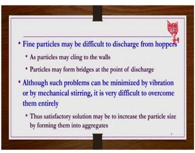
Now we have also seen that fine particles may be difficult to discharge from hoppers because sometimes they may be clinging to the wall surface of the container and then forming a kind of bridges as I already drawn a picture and shown a hopper something like this, you may be having fine particles filled over here entirely. So then what happens you know the fine particles may be sticking to the walls, you may not be able to discharge them properly like this.
