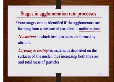
Then stages in agglomeration rate processes, what stages in general you have? In general there are four stages are possible. Four stages can be identified if the agglomerates are forming from a mixture of particles of uniform sizes. That is uniform mixture that you have, so from that uniform mixture of fine particles if you take and then you do a kind of agglomeration so you may find the agglomerates in four stages. What are those stages? We see now.
