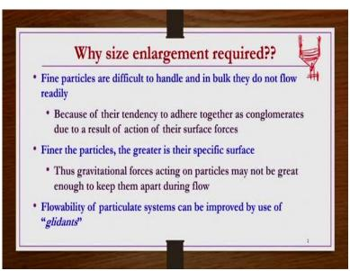
So why size enlargement required? Because fine particles we understand that there are very difficult to handle and in bulk they do not flow readily, that is what in general we have seen. Even in the previous modules, in the storage and conveying section also we have seen, if the
