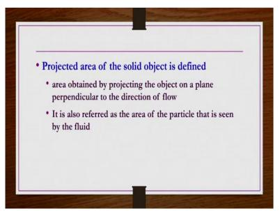
So now projected area or the solid object how to define this? It is defined as the area obtained by projecting the object on a plane perpendicular to the direction of flow. So, that is how the projected area is defined. Or, it is also referred as the area of the particle that is seen by the approaching fluid. So, now pictorial we see some examples. Now we take a projected area of a sphere that we try to calculate. So, we try to calculate now projected area for different objects.
