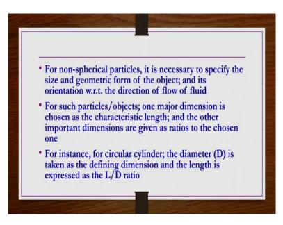
For non spherical particles, it is necessary to specify the size and geometric form of the object; and its orientation with respect to directional flow of fluid. For such particles objects one major dimension is chosen as the characteristic length; and the other important
