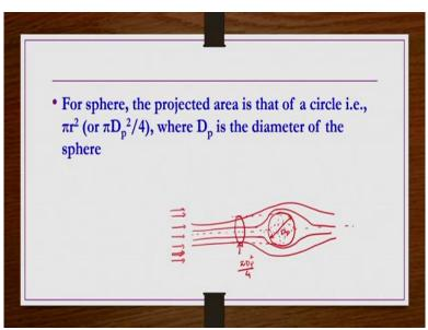
So, we take a kind of spherical object let us say like this. So, now from here the fluid element is coming or the approaching fluid is coming from this direction. So, when this flow comes here it is here depending on the holes small or large is the magnitude of this fluid. The velocity steam lines flow steam less we can have different shapes like this. So, now the projected area of this solid sphere solid spherical particle is the area that you can see from the flow direction.
