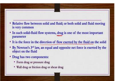
And, then we know by newton's 3rd law an equal and opposite net force is exerted by the object on the fluid. So, whatever the drag force let us say fluid is exerting a drag force of 10 newtons on the kind of solid object.
