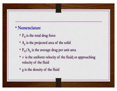
F<sub>D</sub> is the total drag force that is you know fluid is exerting on this solid object and the A<sub>P</sub> is the projected area of the fluid. Projected area we are going to see now and then  $F_D/A_p$  is average that per unit area of the surface and then V is the uniform velocity of the fluid or approaching velocity of the fluid. And  $\rho$  is the density of the fluid.
