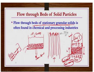
Why because, flow through beds of stationary granular solids is often found in chemical and processing industries in large number of applications. Let us say we have a kind of column in general like this and then at the bottom of the column there is a kind of perforated plate. So, this plate is having some kind of perforation, right. So, now these particles whatever the particles that you know we want we are using them as a kind of a packing and they are placed on this perforated plate.
