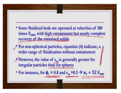
So, fluidized beds are operated at velocities of 100 times, minimum fluidization velocity with high entrainment, but nearly complete recovery of the entrained solids. Sometimes you know, if you are not worried about the entrainment of the solids, because you are sufficiently able to recover them and then send back to the bed so, that you can have a circulating fluidized bed, so under such conditions some fluidized beds are even you know operated at 100 times the
