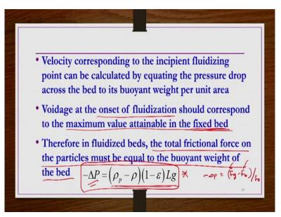
So, velocity corresponding to the incipient fluidizing point can be calculated by equating the pressure drop across the beds to its buoyant weight per unit area and then voidage at the onset of the fluidization our incipient point of the fluidization should correspond to the maximum value attainable in the fixed bed conditions, okay, in the fixed bed conditions. Therefore, in the fluidized bed, the total frictional force on the particles must be equal to the buoyant weight of the bed.
