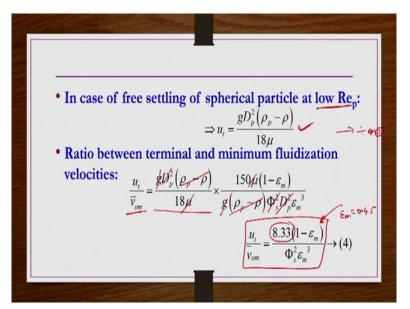
Now, what we do, we try to see the free settling velocity of a single particle and then compare with the kind of minimum fluidization velocity for smaller Reynolds number conditioned. So, small Reynolds number conditions when Re<sub>p</sub> is less than one we have already seen for spherical particle free settling velocity is nothing  $\frac{gD_p^2(\rho_p-\rho)}{18\mu}$ .
