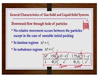
Let us say a general characteristics of gas solid and then liquid solid system and under such conditions we take a downward flow through beds of particles. Okay, what we have? We have the kind of column as I mentioned already, right. So, this column is packed with some kind of particle backing material. So, we have different types of packing materials also those things also we have seen.
