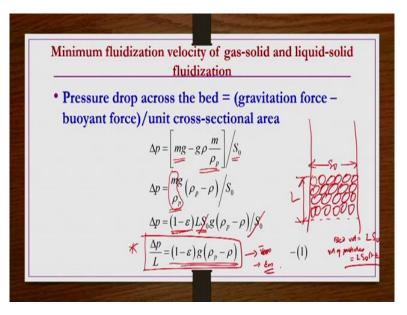
So, minimum fluidization velocity of gas-solid and liquid-solid fluidization. Remember up to the fluidization incipient fluidization are the minimum fluoridation conditions whether the fluidizing medium is a gas or liquid it is going to be here kind of a similar way. So, whatever the minimum fluidization velocity calculations are there, they are going to be same whether the fluid is a medium is a gas or liquid, okay.
