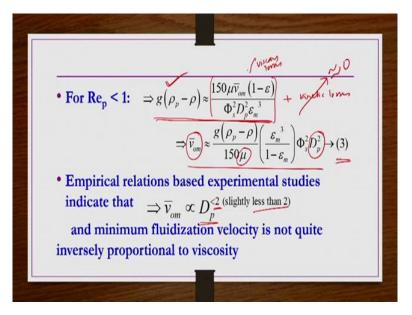
So, now, in the case of single particle conditions, a single particle settling in a column of fluid if we know the Reynolds number, so, then we have a kind of you know expression for a free settling velocity of the that particular particle. If we know that the particle settling under the Stokes regime then we have a kind of free settling velocity for that particle under Stokes regime.
