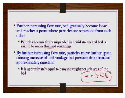
Further increasing the flow rate, bed gradually become loose and reaches a point where the particles are separated from each other. And then particles become freely suspended in liquid stream and then bed is said to be under fluid as to conditions. The same thing we are going to see pictorial in the next slide anyway.
