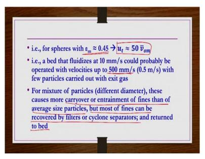
That means, resettling velocities almost 50 times the minimum fluidization velocity. So, if your velocity, whatever you are going to provide for the you know minimum fluidization to take place at least minimum fluidization to take place. So, it has to be at least 50 times the free settling velocity of the single particle. You find out what is the free settling velocity of
