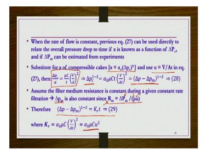
When the rate of flow is constant, the previous equation number 27 can be used directly to relate the overall pressure drop to time if alpha is known as a function of  $\Delta p_c$ , and if  $\Delta p_m$  can be estimated from experiments. So in that above equation substitute  $\alpha = \alpha_0 (\Delta p_c)^S$  and use u = V/At in equation number 27. So this is your equation number 27.
