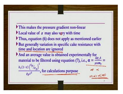
And because of that one, the pressure drop or pressure gradient becomes a kind of non-linear. And then local value of  $\alpha$  may also very with time in general. Thus, whatever the equation number 6 that have been developed for cake resistance does not apply as mentioned earlier for a case of a compressible cakes that can be applied for incompressible cakes. But for compressible cake that is not applied.
