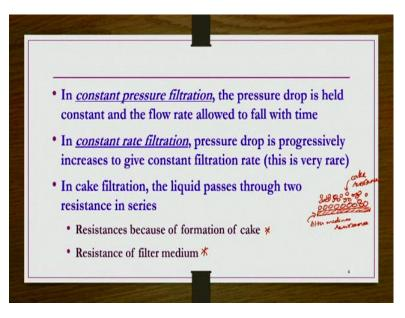
In constant pressure filtration, the pressure drop is held constant and the flowrate allowed to fall with time. In constant rate filtration, that is constant volumetric filtration rate. If you maintain constant volumetric filtration rate, the pressure drop is progressively increases to give constant filtration rate. But however, this is a very rare case.
