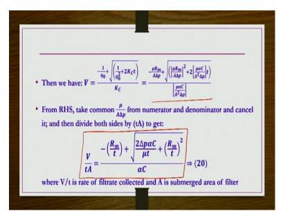
So, if you substitute them here in this equation, equation number 19 then we have this equation. From this equation, what you do? You take  $\frac{\mu}{A\Delta p}$  common from the both numerator and denominator of the right-hand side and strikeout. And then after that step you divide both sides
