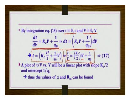
Okay, so by integration equation 15 over the limits t is equal to 0 to some instant t and then volumetric flow rate initially it is 0 anyway. At time t if volumetric flow rate or volume of filtrate collected is V, then if you use them as a kind of limits, then this equation number 15 is this one, you integrate this one. So integration for that purpose dv you take to the right inside.
