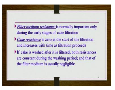
In general filter medium resistance is normally important only during the early stages of the cake filtration. Because you know what happens as the time of filtration gradual increases, more and more number of particles are depositing on the surface of the filter medium. And those particles are forming a kind of cake and that cake is offering much more resistance compared to the whatever the filter medium resistance is there.
