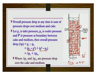
Now, what we understand from here? There are two resistance, so then obviously there will be a kind of two pressure drops. So the overall pressure drop at any time is going to be sum of pressure drops over the filter medium and across the cake formed. That cake formation or whatever the cake has form, across that cake form, whatever the pressure drop is there that one, plus the pressure drop across the filter medium.
