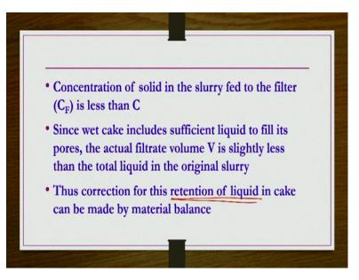
Let us assume, concentration of solid in the slurry fed to the filter is  $C_F$  and that is less than C okay. Because wet cake includes sufficient liquid, to fill its pores, then actual filtrate volume V is slightly less than the total liquid in the original slurry. Because the entire liquid is not coming as a kind of filtrate, some amount of the liquid is retained interstitial space between the particles whatever is there within the cake.
