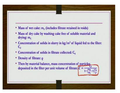
How it can be made? Let mass of wet cake is mf, which includes the filtrate retain the voids or the liquid that is retained inside the or between interstitial spaces of particles within the cake. And then mass of dry cake that is after washing the cake, free of soluble materials and drying it, whatever the mass is there that if you take mc.
