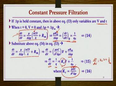
Okay, so now, so that equation, we have this basic equation, whatever have  $\frac{dt}{dv} = \frac{\mu}{A\Delta p} \left(\frac{\alpha CV}{A} + R_m\right)$ . If you operate, or if you use this equation for constant pressure filtration. Then you have a kind of a methodology to calculate this  $\alpha$  in Rm.
