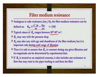
Now filter medium resistance, analogous to cake resistance  $\alpha m_c/A$ , the filter medium resistance can also be defined as  $R_m = \frac{\Delta p_m}{\mu u}$ , where  $\Delta p_m$  is nothing but  $(p' - p_b)$ . Here typical values of Rm in general ranges 10<sup>10</sup> to 10<sup>11</sup>. So now we have a expressions in terms of a maybe pressure drop, we have expression for the cake resistance as well as the filter medium resistance, okay.
