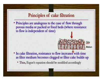
So, in cake filtration we have seen. Like you know there is a kind of filter medium onto which like you know normal to the surface of the filter medium. The slurry is allowed to pass through and then whatever the coarse particles, large amount of coarse particles are there. There will be forming a kind of a layer, which forms a kind of a layer of particles which is known as a kind of cake, cake formation.
