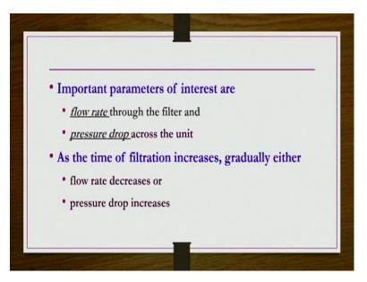
So in this cake filtration, what are the important parameters of interest? Obviously we have seen that the filtrate, the volumetric flowrate and then resistant to the flow. That is the pressure drop and that increases right. That pressure drop increases with time. So these are the kind of two important things. So these are flowrate through the filter and pressure drop across the unit okay.
