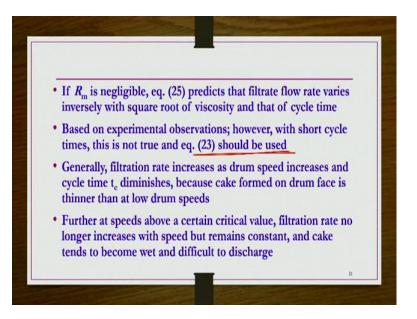
So if Rm is negligible, equation 25 predicts that filtrate flow rate varies inversely with square root of viscosity and that of cycle. But in general, that is not true based on the experimental observations; especially, for short cycle times, this is not true and then equation 23 should be used, okay.
