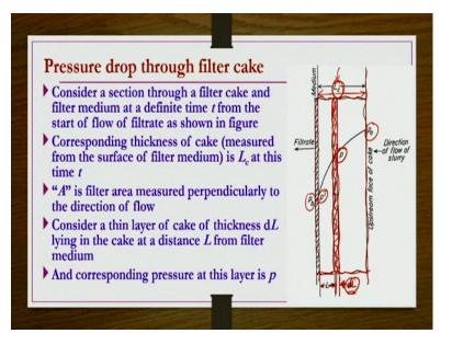
Now, you wanted to calculate this pressure drop of through the filter cake. Because these pressure drop equation for. Now this cake is behaving as a kind of, you know, almost kind of a packed bed kind of thing. And then for the packed bed pressure drop equations, you are having. So one way or another way you can make use of that flow-through packed bed cases for which whatever the pressure drop equation is there.
