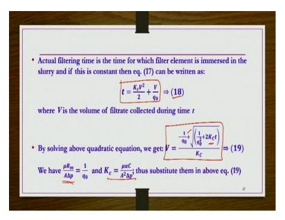
What are those modification? Actual filtering time is the time for which filter element is immersed in the slurry and if this is constant then equation 17 can be rewritten as like this that whatever the  $\frac{t}{V}$  was there, what V was there in the left-hand side that has been taken to the right-hand side and then given equation number 18. So that  $t = \left(K_c \frac{V^2}{2} + \frac{1}{q_0}V\right)$ .
