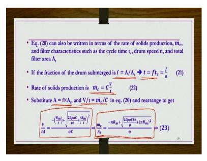
So this equation 20 can also be written in terms of the rate of solids production, mc and then filter characteristics such as the cycle time  $t_c$ , drum speed n, and total filter area  $A_t$  etc. So, if the fraction of the drum submerged is f then  $A/A_t$  is nothing but f. Then cycle time, we can write  $ft_c$  is nothing but the t, which we can also write as f/n. That is the n is nothing but drum speed.
