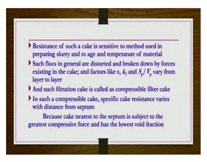
However, resistance of such a cake is sensitive to method used in preparing slurry and the age of slurry and temperature of material, which has been you know applied for the separation or required of filtration process. Such flocs in general are distorted and broken down by forces existing in the cake; and factors like  $\varepsilon$ ,  $k_2$  and  $\frac{S_p}{V_p}$  in general vary from layer to layer. Because of that one pressure drop is also going to be non-linear.
