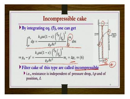
So now, incompressible cake. So these cakes are in general can be compressible or incompressible cakes, whatever the cake resistances is there, that is independent of the pressure drop and then that is not going to change with change in the L. Then we can call such cakes are kind of incompressible cake. But in general, most of the cakes are in compressible only. So we see both what is incompressible cake and then compressible cake right now.
