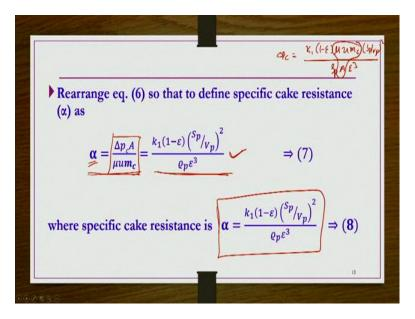
Now, if you rearrange equation number 6, so that to define specific cake resistance. So actually, we now coming to the position where we can describe or develop equation for two different resistance that we have. We have two resistance for the cake filtration cases, one is the cake resistance, another one is the filter medium. So we have arrived to a kind of point, where we can measure the cake resistance.
