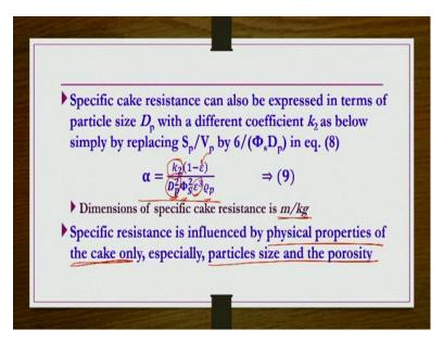
But in general, specific cake resistance can also be expressed in terms of particle size Dp with the different coefficient  $k_2$  as below by simply replacing  $\frac{S_p}{V_p}$  by  $\frac{6}{(\varphi_s D_p)}$  right. So then we get  $\alpha$  is equal to that constant will be modified that, you know whatever 4.17 is there, now here that  $6^2$  is also there right. So that whatever the new thing is coming, constant is coming that we can call it as  $k_2$  okay.
