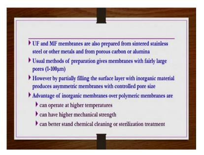
Then ultra-filtration and micro filtration membranes are also prepared from sintered stainless steel or other porous carbon or alumina as well. Usual methods of preparation gives membranes with fairly large pores varying from 1 to 100 microns, 1 to 100 microns is a very wide pore size distribution, so in general that is not good for a given application. So, it is better to have a pore size distribution narrower. So for that in general what you do? You can have a kind of partially
