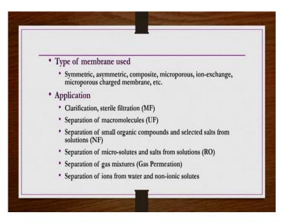
And then types of membranes used, different types of membrane processes. Different type of membranes are used, like sometime symmetric membranes are good, sometimes asymmetric membranes are good, like that in composite, micro porous, ion-exchange, micro porous charged membranes, etc. are also available so what type of membrane are we using, that is also going to have a significant role in the membrane separation process.
