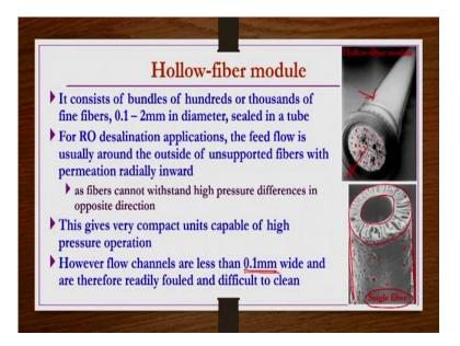
The last module is the hollow fiber module. Here what we have, it consists of hundreds or thousands of fine fibers, which are having the diameter in general, 0.1 to 2 m, they are sealed in a kind of tube. There are fibers, large numbers of such fibers which are of small size are taken in hundreds and thousands, in general, and they are packed in general in a tube, we will see pictorially as well.
