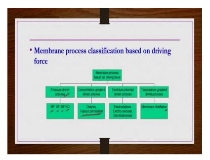
Then membranes process classification based on driving force. As we have seen the separation is occurring based on the, you know, type of driving force applied. So it is possible that when a particular type of driving force is applied, whatever the membrane processes are there, they may be designated as a kind of or named as a kind of certain membrane processes. So, based on the driving forces how we can classify these membrane forces that we are going to see now here.
