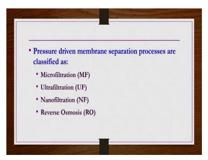
In this lecture we will be discussing only those separation processes which are based on the pressure gradient driving force, why because whatever the filtration those things we have been seeing, we are primarily considering only the pressure based, or you know vacuum based, or centrifugal force based filtration processes only we consider which are better for a filtration process. So, membranes there are several types of driving forces are there.
