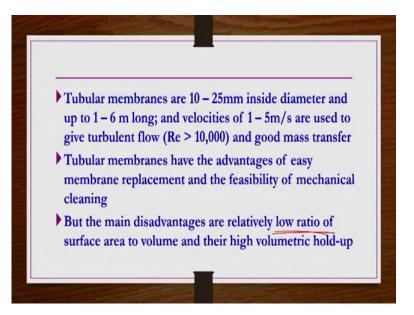
So tubular membranes or whatever the tubular modules, whatever the membranes are used usually 10 to 25 mm inside the diameter and up to 1 to 6 m long and velocities can be as high as 1 to 5 m/s which correspond to the turbulent flow where Reynolds number is greater than 10,000 in general because of that one good mass transfer would be there. Tubular membranes have the advantages of easy membrane replacement and feasibility of mechanical cleaning.
