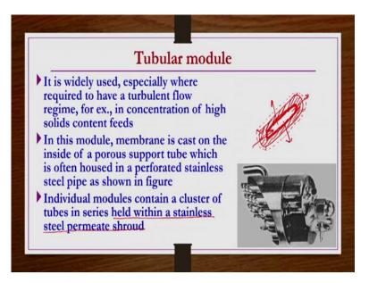
In tubular modules they are in general widely used specially where required to have a turbulent flow regime or you know like you know concentration of high solids content feed, etc. then this tubular modules are used. So what are these tubular modules, in this tubular modules membrane is cast on the inside of the porous support tube, what we have a kind of a porous support tube is, this tube is having a kind of a porous structure, right.
