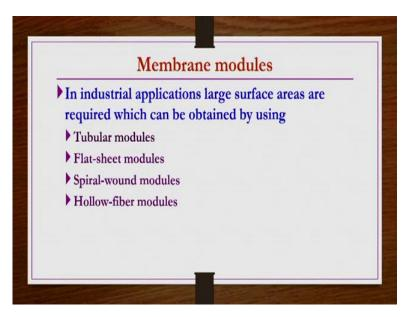
In industrial applications large surface areas are required which can be obtained by using tubular modules, flat sheet modules, spiral wound modules and hollow fibre modules, we see a few details of each of this four modules now.
