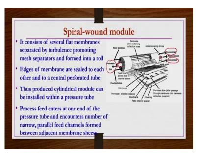
The next one is the spiral wound module, so here it consists of several flat membranes separated by turbulence promoting mesh separators formed into a roll. Edges of membrane are sealed to each other and to a central perforated tube, thus produced cylindrical module can be installed within a pressure tube. Process feed enters at one end of the pressure tube and encounters number of narrow parallel feet channels found between adjacent membrane sheets.
