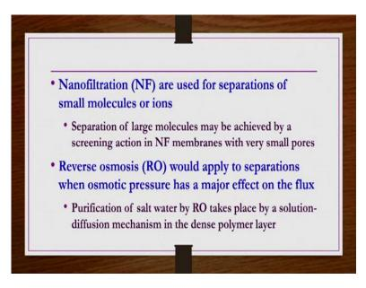
Whereas the nano-filtrations are used for separation for small molecules or ions, separation of large molecules might be achieved by the same nano-filtration where the screening action takes place using a kind of nano-filtration membranes with very small pores. In general, nano-filtration membranes are used or nano-filtration separation processes are used to separate very small molecules or ions.
