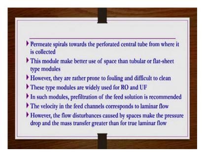
Then permeate spirals towards the perforated central tube from where it is collected. This module makes better use of space than tubular or flat-sheet type modules that we have seen. So, that means we can have a kind of a higher capacity operations with this kind of modules. However, they are rather prone to falling and difficult to clean in general. These type modules are widely used for reverse osmosis and ultrafiltration.
