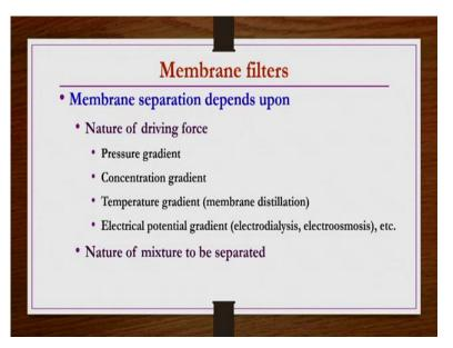
So, then membrane filters and how to classify them. Membrane separation depends upon nature of driving force that we have seen. So, given type of separation you need to find the appropriate driving force. According you need to do, if only one driving force is required, if more than one
