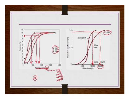
So, now we see couple of pictures about the molecular weight cut off. Now here in this first picture what we can see, we can say x axis molecular weight of PEG that means you know these are the different solutions, PEG solutions are prepared which are PEG of different molecular weights are taken like you know 100, 500, 1000, 10,000 like this, you know, up to 1 lakh molecular weight or even more are available.
