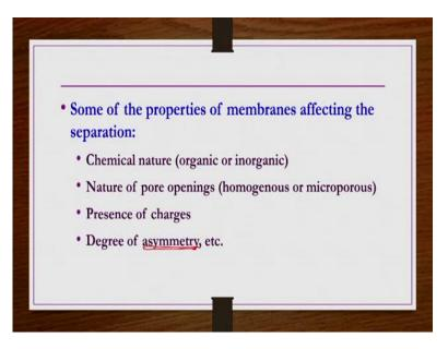
Now, we understand that you know the properties of membrane are definitely going to show a kind of effect on the separation process because depending on nature of the membrane, depending on charges, etc. there on the surface, you know definitely some of the properties, even depending on the pore structure; how narrow pore sizes are, how wide range of pore structure are there; depending on that one also the separation process is going to be affected.
