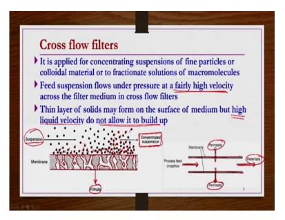
So what is Cross flow filters? As we have already seen the basics of filtration process, Cross Flow filtration: where we have a kind of a, a kind of membrane as a kind of a filter medium. So, this membrane may be having a kind of a porous structure, which may be a kind of almost channel kind of a structure or which may be having a kind of a connecting porous structure, something like this shown here, right? So, some of the channels openings are connected to the other porous openings.
