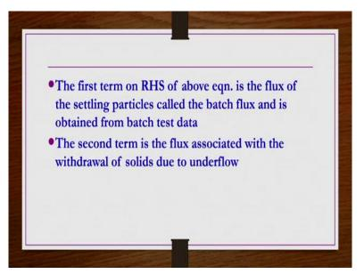
So the first term of RHS of the above equation is the flux of the settling particles called the batch flux, that is c cv is nothing but the batch flux and is obtained from the batch test data. The second term is flux associated with the withdrawal of the solids through the bottom due to underflow that is known as a kind of underflow flux.
