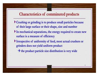
Now characteristics of comminuted products. Crushing and grinding is to produce small particles because of their large surface or their shape, size and number as well. Sometimes, that is the reason we do crushing or grinding crushing and grinding are some kind of a size reduction operation. Okay, so we are doing the size reduction operations to produce small particles.
