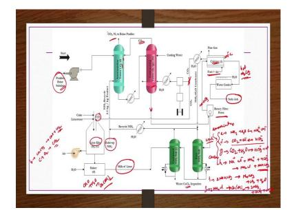
Now, this is the flow sheet that we have having here. So, purified brine solution whatever is there that is pumped to a ammoniation tower where reactions e and then f are taking place, right. So, where this reaction is e is nothing but ammonia reacting with water to get ammonium hydroxide. Actually, they are produced in you know such a way that they can be easily decomposed and then it is a reversible reaction.
