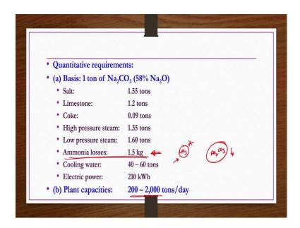
Quantitative requirements basis 1 ton of sodium carbonate that is 58 percent Na 2 O, salt 1.55 tons, limestone 1.2 tons, coke 0.09 tons, high pressure steam 1.35 tons, low pressure steam 1.6 tons, ammonia losses 1.5 kgs, cooling water 40 to 60 tons, electric power 210 kilo watt hour. Ammonia losses also it has to be carefully designed and then utilized because you are using ammonia which is expensive to produce a low cost chemical like you know sodium carbonate.
