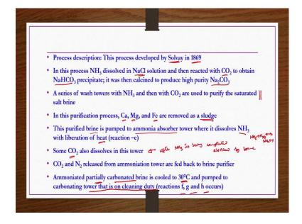
Now, the same process we are going to discuss as a description part. This process developed by Solvay in 1869. So, because of him this process is also known as the Solvay process which is also has nothing but ammonia soda process. In this process ammonia dissolved in sodium chloride solution and then reacted with CO 2 to obtain sodium bicarbonate precipitate it was then calcined to produce high purity sodium carbonate.
