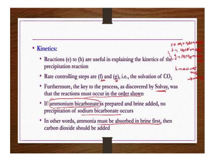
Kinetics: reactions e to h are useful in explaining the kinetics of the precipitation reaction because e to h reactions e to e reaction we have already seen ammonia reacting with water to give ammonium hydroxide reversibly.
