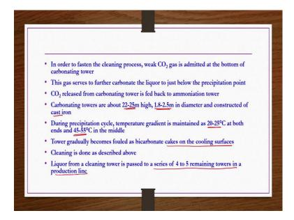
In order to fasten the cleaning process weak CO 2 gas is admitted at the bottom of carbonating tower. This gas serves to further carbonate the liquor to just below the precipitation point. CO 2 released from carbonating tower is fed back to ammoniation tower. Carbonating towers are about 22 to 25 meters high and then 1.8 to 2.5 meters in diameter and they are constructed of cast iron.
