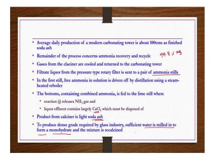
Average daily production of a modern carbonating tower is about 100 tons as finished soda ash remainder of the process concerns about the ammonia recovery and the recycle. Remember this process is not going to be effective if you are not effectively recovering the ammonia. What do you mean by effectively recovering ammonia?
