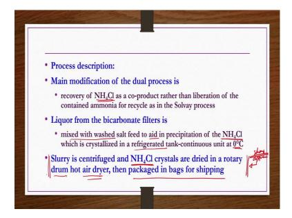
Process description main modification of the dual process is recovery of ammonium chloride as a co-product rather than liberation of the contained ammonia for recycle as in the Solvay process, liquor from the bicarbonate filter whatever is there that we in the initial Solvay process react with the calcium hydroxide to get ammonia, but here we are not doing that one.
