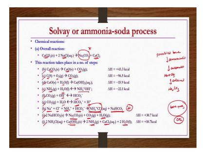
Solvay or ammonia soda process: chemical reactions of this process would be discussed first. Overall reaction, calcium carbonate reacts with the sodium chloride to give product, sodium carbonate and then ways to take dispose of that is calcium chloride is also produced.
