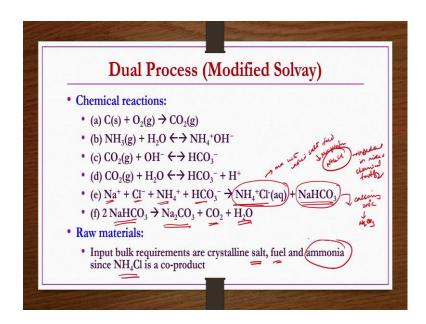
Now, we discuss about the modified solvay process or dual process, ok. So, in this modified process what we do? Rather reacting ammonium chloride with calcium hydroxide to give ammonia and then recycling, what we are doing? We do mixing of this ammonium chloride with a salt and then we try to do the crystallization by refrigerating it at 0 degree centigrade continuously so that you can also have ammonium chloride as co-product in the production of sodium carbonate, ok.
