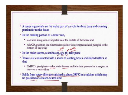
A tower is generally on the make part of cycle for three days and cleaning portion for twelve hours because that sodium carbonate is continuously forming as a cake on the walls of the towers. So, that has to be scrapped continuously. Whatever continuously you are scrapping or whatever effectively you are scrapping that sodium bicarbonate precipitation from the walls of the tower, there is still a requirement of cleaning.
