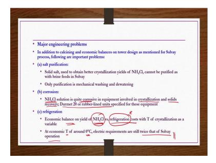
Major engineering problems: in addition to calcining and economic balances on tower design as mentioned as mentioned in Solvay process that we have just discussed following are important problems. One is the salt purification. Solid salt used to obtain better crystallization yields of ammonium chloride and cannot be purified as with a brine as with sodium chloride brine feeds in Solvay process only purification is mechanical washing and dewatering is possible.
