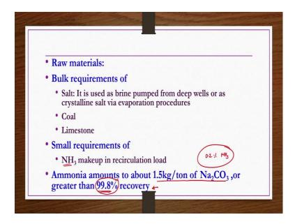
Coming to the raw materials obviously, bulk requirements of salt it is used as brine pumped from deep wells or as crystalline salt via evaporation procedures. Then coal is required because you need CO 2, then limestone is required because you have to decompose the ammonium chloride to get the ammonia and then calcium chloride. So, for that purpose this limestone is required and then small requirements of ammonia makeup in re-circulation load is also there.
