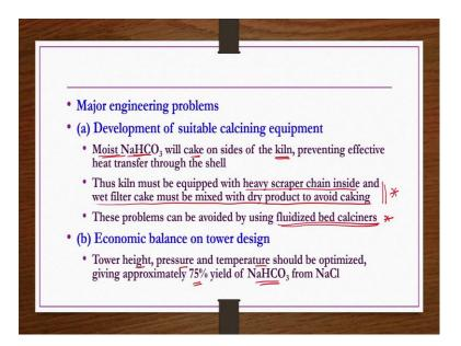
Now, we see major engineering problems: development of suitable calcining equipment. Sodium bicarbonate is in the wet condition actually that is being calcined to get the sodium carbonate. So, this calcining you will be doing in a kilm, right. So, that on the walls of the kilm this cake formation may be taking place.
