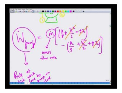
But, theoretically speaking what is the rating of a pump for a given application in order to do this you have to just write the energy balance across the inlets and exists of a pump. So, the rate at which pump does work W dot pump is m dot times p 1 by rho plus V 1 squared by 2 plus g z 1 minus p 2 by rho plus V 2 square by 2 plus g z 2, this is the mass flow rate.
