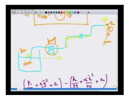
I can write therefore, h l is nothing but, f times half head loss in a pipe half V square L by D divided by g, this is the relation between the friction factor and the head loss in a pipe, this is the relation between the friction factor and head loss in a pipe.
