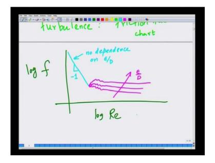
So, you have plotting f verses R e for different values of epsilon by D. So, in the laminar regime, so this is in a sense in a logarithmic plot, so it is log f verses log R e double logarithmic plot; so in the laminar regime f verses R e will have in a double logarithmic plot as slope of minus 1 because, f is inversely proportional to Reynolds number in the turbulent region it is not very clear.
