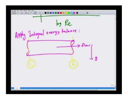
Now, once we know the friction factor then, we can estimate what are the head losses in a pipe, for that we have to take a pipe a straight pipe. So, gravities are acting perpendicular to the direction of flows, so the flow is in this direction and you apply energy balance, macroscopic integral energy balance, when we do that, we take the stations of the control volume 1 to be like this and 2 to be like this.
