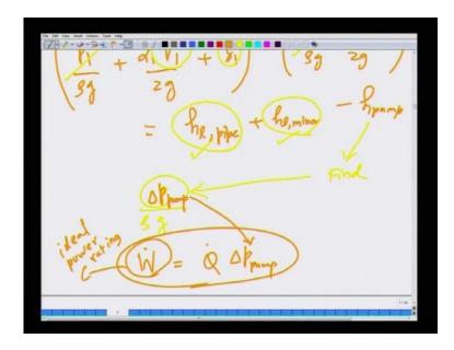
h pump is nothing but, delta P by rho g, now once you know what is delta P once you know h pump you can find delta P, once you know delta P then, the rate at which work must be done by the pump on the fluid is nothing but, Q dot times delta P, this is delta P across the pump and if you take this delta P you can find the horsepower rating of the pump.
