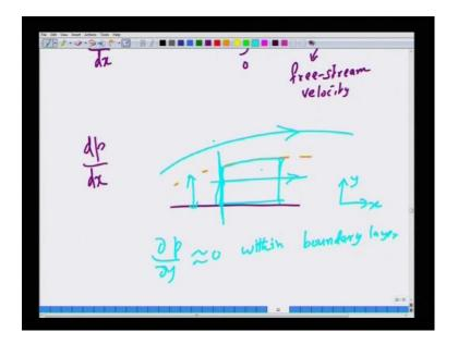
Minus delta d p d x minus tau w after dividing by w d x in the entire expression is d d x of integral 0 to delta of x rho u square d y well for minus u integral d d x of integral rho u d y, capital U is the free stream velocity outside the boundary layer, velocity and that is outside the boundary layer.
