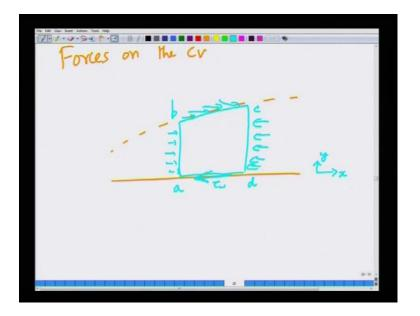
So, this is nothing but, minus U partial by partial x of integral 0 to delta rho u d y d x times w, now what are the forces, because you have to now worry about the forces on various phases, there are pressure forces and there are shear stresses, exerted by the solid surface; forces on the c v, so we have to now worry about what are the forces on the c v.
