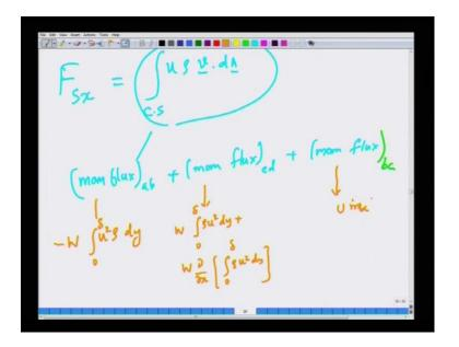
So, we will first focus on this term is equal to the momentum flux through a b plus momentum flux through c d plus the momentum flux due to b c, there are these three phases through which momentum come in by virtue of flow a d c d and b c, these are three phases and the bottom phases is informable, so there is no momentum flux (Refer Slide Time: 36:32).
