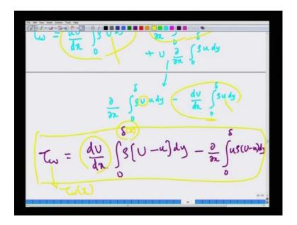
Now, I am going to split the last integral in the following way, now I am going to write this as d d x of integral 0 to delta rho U u d y minus d U d x of integral 0 to delta rho u d y, the last integral can be written like this by product rule, because both U and delta are functions of x, so here U is out, so I am bringing u in but then now I have to subtract and equivalent this is just product rule of 2 multiplication of two functions.
