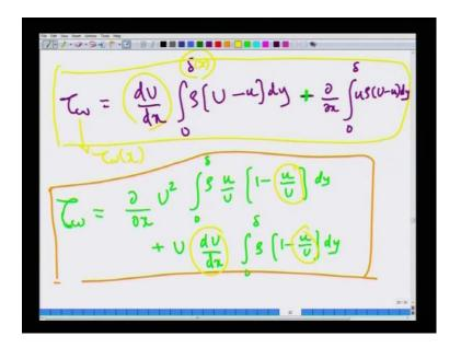
So, tau w is partial by partial x of U squared of integral 0 to delta rho u divided by U times 1 minus u divided by U, all I am doing is to take this u out and then I write d d x of d u d x as d d x of u square 1 minus u by u d y plus I am sorry there as to be plus sign here, because I am using capital U first, so capital U is multiplied by plus here.
