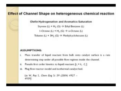
Now, there is some very interesting and the interesting application I should say of the conduit shape on heterogeneous chemical reactions of both fast and slow reactions and in micro systems or milli systems, this is particularly with reference to monolith reactors which are very popular in automatic as a reactor cases and in the next class, we will be discussing how the channel shape influences the heterogeneous chemical reactions and how this helps us in a proper design of micro reactors.
