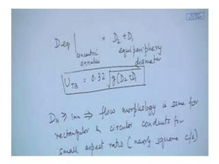
The people have found that the proper equivalent diameter for a concentric annulus is not the hydraulic diameter incase of Taylor Bubble rising, but it is actually they have called it as an equi periphery diameter and this explains the phenomena that we have to see, that the rise velocity of the Taylor Bubble it increases both with increase in the dimension of the inner as well as the outer tube. With this particular definition the rise velocity expression becomes as shown well.
