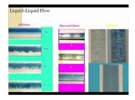
Now suppose instead of air water, I introduce may be an oil; it can be kerosene, it can be towline, it can be anything. I introduce another oil, do we expect the same flow patterns to exist? See one thing is for sure gravity, in this case also will be trying to pull the lighter phase towards the top, heavier phase towards the bottom.
