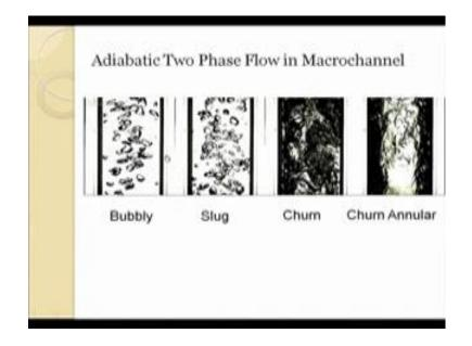
Now, this particular case if you find; we find that due to the highest surf extension of the liquid, it cannot assume the shape of the elongated plugs as we observed in gas liquid cases; on the contrary when the waviness is very much, then it shreds the interface.
