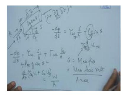
Suppose we are having may be say we consider delta z portion or delta z length of the pipe of cross sectional area A and here we find and may be the wetted perimeter as S. In this particular case, the pressure is going to or the pressure force is PA and in this particular case, we find that, the pressure force is P del P del Z into delta Z into A and here we find that the gravity is acting and there is a component in this particular direction.
