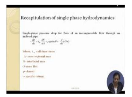
Then what do we get, we get a pressure drop relationships. I leave it as a home assignment, to perform this particular balance and then finally, arrive at an expression to find out the pressure gradient. This expression is TW the S by A plus say row G pipe inclined, then have a sign theta component; where theta is the angle where horizontal plus this gives you d d z of u into say G.
