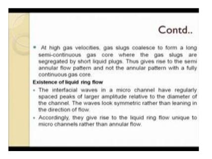
Again at higher gas velocities what we found was, the gas slugs they are coalesce to form a semi continuous gas core; where the gas slugs they were separated by short liquid plugs.
