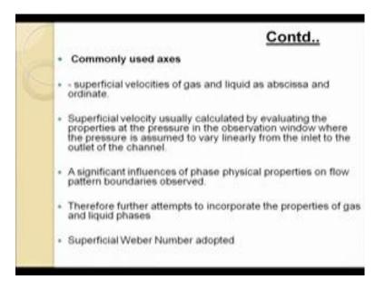
In this way the flow patterns are identified, and the flow pattern maps were made. In this case also we find that the commonly used axes of superficial velocities of the gas as
