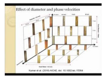
And this also 3 dimensional flow pattern map, that we are try to develop just in order to show the coupled effect of liquid velocity, gas velocity and pipe diameter.
