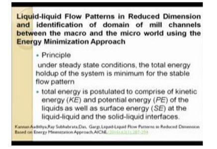
With this more or less I have given you idea regarding the basics of the flow pattern in a micro channel, the flow pattern maps now I would want to discuss one particular analytical model based on basic physics which we have developed in the multiphase flow laboratory to predict the liquid-liquid flow patterns in reduced dimensions, we have used for liquid-liquid flow, but it its more or less general it can be used for gas liquid flow in reduced dimensions as well.
