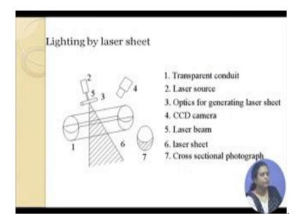
Well there is one more thing also to capture the cross section we can have we can generate a laser sheet as shown in the particular slide and this particular laser sheet enables its illuminates the cross section and gives us an idea regarding the cross section
