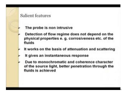
Now, the some of the salient features of the probe which explains it is versatility or popularity is firstly, it is non intrusive secondly, the detection of the flow regime does not depend upon the physical properties like corrosiveness of the fluids.
