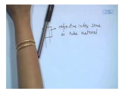
Or a square box which is installed in the in the section which you want to view and this particular box is usually filled up with some particular material which as the same refractive index as the refractive index of the tube material refractive index same as tube material.
