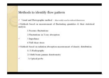
In fact, the most widely used technique as I have told you the visual and photographic method they actually operate on the difference in the transference of the optical property of the 2 phases and this is the method which is most widely used.
