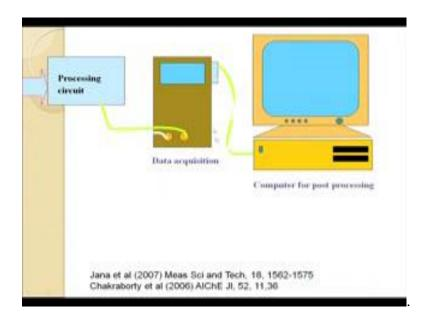
And there is a photo diode sensor at the top this photo diode sensor when it receives light it converts it into a voltage signal and then this voltage signal is send to a processing circuit for further processing and data acquisition and then it gives us a continuous voltage time signal on the computer screen by means of each we can understand flow distribution.
