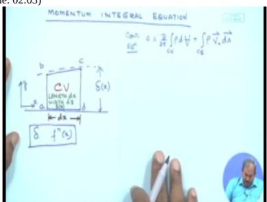
start with the continuity equation which we have derived which simply tells me that this would be the form of the continuity equation and the moment we assume that it is a steady
