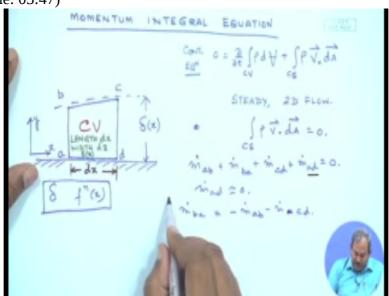
the continuity equation with which we are going to proceed. Now surface a b is located, surface a b is located at x. The location, this location is x and this is x plus d x. So let's see
