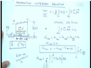
So m dot a b essentially tells me the mass flow rate of, mass flow rate coming in to the control volume through the surface c v. Now when we try to get whatever be the a and b, understand that m dot a d is equal to zero.
