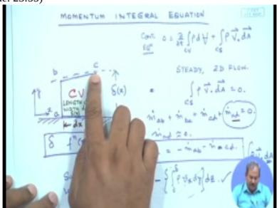
near b c? So if you think of the x component it's zero here, it keeps on increasing and when it reaches the edge of the boundary layer, at the edge of the boundary layer the velocity would simply be equal to the free stream velocity which is U, with which the velocity is flowing outside of
