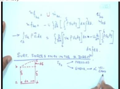
the velocity gradient near the edge of the boundary layer is essentially zero because at or near
