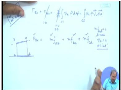
So m f a b when we talk about surface a b, m f a b would simply be equal to minus of zero to delta  $v \times v$  rho  $v \times v$  d y d z.
