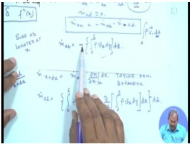
negative sign whereas m dot c d the sign is going to be positive. So once I have analytically what is the, what is the expression for the mass which comes in through the surface a b,
