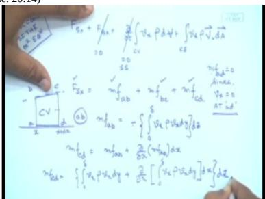
So entire this thing, first term del del x of this multiplied by d x and d z where d z is the direction perpendicular to this. So I now have m dot m f a b, I have m f c d. I need to find out what is m f b c. Now m f b c, m f b c would be equal to, I know what is the expression for m dot b c from my previous, previous analysis we have seen that m dot b c is simply this term
