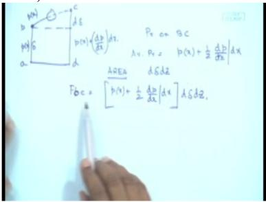
force on b c, force on b c is the average pressure multiplied by the projected area of b c in the x direction this is the x direction so it is d delta times d z where d z is the depth. So whatever be the average pressure multiplied by d delta d z would give me the f f b c force on it. The only thing which is remaining is f, force on a d and we understand that force on a d is equal to shear force only. It's a shear force only
