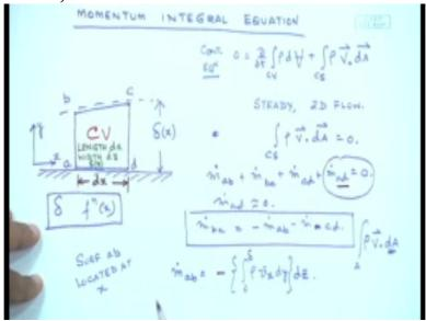
Let's concentrate on the other surface which is m dot c d. m dot c d is located at the distance d x from a b where a b is located at x and c d is located at x plus d x where d x is small. So the function m dot a b, if we take Taylor series expansion of the, of this m dot a b and disregard all the higher order terms then
