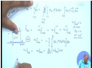
so therefore m f c d would be equal to this. However you understand, you see that since momentum is leaving the surface c d therefore it's going to be positive and since momentum is coming into c v through surface a b therefore m dot a b is negative, same convention as
