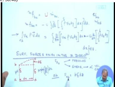
due to pressure which can be expressed as the local value of pressure multiplied by the local value of the boundary layer thickness and the depth of the flow field. What is going to be at the surface c d? On surface c d, f c d would simply the pressure is going to be p plus d p d x multiplied by d x and delta has also changed delta has become delta plus d delta and d z will remain unchanged. So
