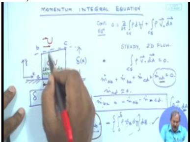
the boundary layer. So to the expression of m dot b c, I must multiply with u, the x component of velocity near b c to obtain what is the x component of momentum contribution due to the flow through b c. So m dot b c, the expression for m dot b c
