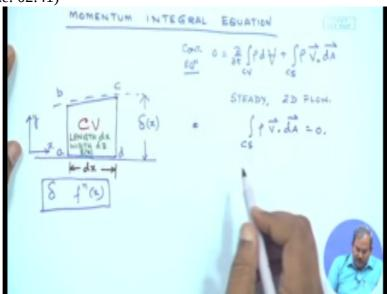
Now this for a control volume which is defined by control surfaces we simply can say that m dot a b plus m dot b c plus m dot c d plus m dot a d would be equal to zero. So the mass flow rate through the surface a b, through the surface b c, through the surface c d and through the surface a d would be equal to zero.
