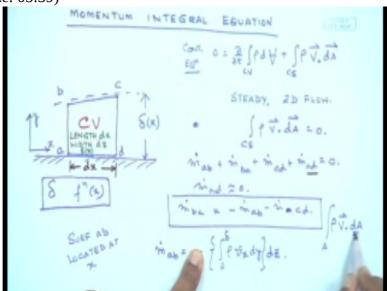
the velocity in this case which contributes to the x, which contributes to the amount of mass which enters is v x, multiply that with rho and what you get is the mass flow rate through the surface a b. However you, you also can see that through the surface a b, mass comes into the control volume. So according to the convention which we have, which I have proposed, which we are going to use
