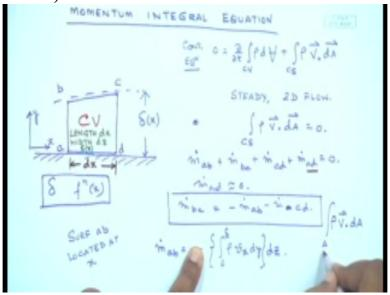
give us the mass so that, that comes in to the control volume. In this case d a is simply d y times d z. So d y times d z is the d a,
