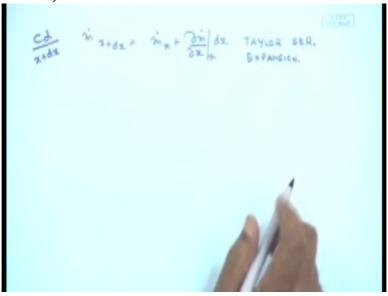
mass product of, through the control surface at c d which is located at x plus d x, I simply take a Taylor series expansion in, in this form by and neglecting the higher order terms. So my m dot c d would simply be equals whatever was m dot x from my previous slide which is rho v x times d y plus del del x zero to delta rho v x d y this is d x and the whole thing is multiplied by d z.
