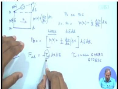
then the force acting on the fluid would be minus of tau w. tau w is the wall shear stress acting on the wall, so the force on the control volume of fluid would simply be equals minus tau w and no pressure force acting on f a d. So what we have done is we have identified, I will
