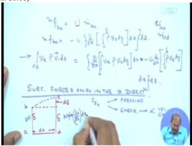
So on one side I have a pressure p x, on the other side, on the other surface c d, the pressure is going to be equal to p plus d p d x. So I have to think of what is the, what is the surface force on surface a b which is, surface a b has only pressure so f a b which is a surface force must be
