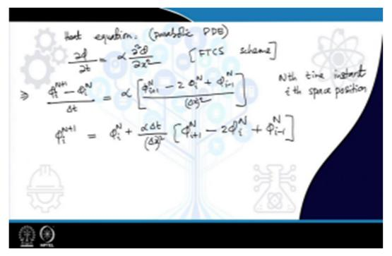
Let us say, so, I am supposed to write down the heat equation which is nothing but a parabolic PDE. So, the left-hand side I will do a forward difference and the right-hand side I will do a central difference. Which is known as, this is known as if FTCS forward in time and central in space. So, let us try to write, I bring down the subscript as well as the superscript to distinguish between the space and time part.
