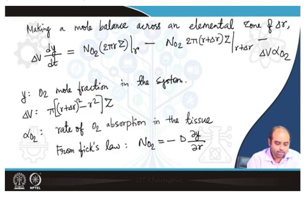
So, making a mole balance across an elemental zone of delta r, we write so this y is the mole fraction of O2, let me write it to you so O2 mole fraction. And delta V is the this elemental volume so which is pi r plus delta r square minus r square Z, of course Z is the length of the
