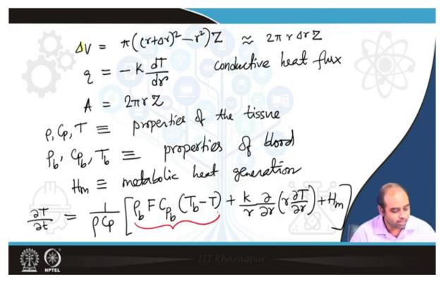
So, here this here delta V is pi r plus delta r so that is the elemental volume multiply with Z, so this is approximately 2 pi r delta r delta Z. q is the from the Fourier law of heat conduction we know that minus K dT dr and only this radial direction heat transfer is considered, so conductive heat flux.
