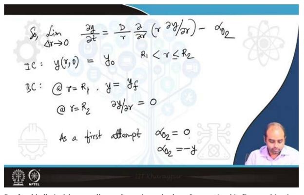
So, for this limit delta r tending to 0 you have dy dt so I can write this D as nothing but diffusivity of oxygen actually. What about the boundary condition? So, the initial condition y r comma 0, t is equal to 0 is let us say this is the initial level of oxygen inside the tissue region, so this of course please note that this r is in between R1 to R2, so it is not from 0 to R2, so it is from the surface of the capillary to the surface of the tissue.
