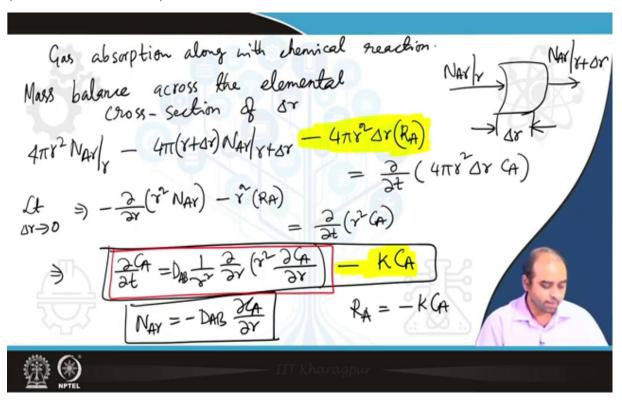
So, in the same context from where we left off in the last class that you have a spherical droplet and the mass transfer takes place by diffusion it is a gas or a liquid droplet dispersed in a liquid or a gas. So, let us try to write this balance equation for the case when we have absorption along with reaction, along with chemical reaction.
