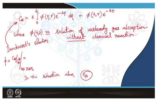
So, let us assume, I mean let us consider that we know the this Danckwert's solution. So, how does it looks like, let me just write you. So, the solution to this case can be written down as this where this phi t comma r is the solution of unsteady gas absorption without chemical reaction and this is something which we have done in the last lecture, we got a detailed solution from the idea of the separation of the variables. So, this is the Danckwert's formula that works in this case.
