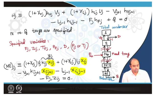
So, for the reboiler, let us also write down for the case of the reboiler, which is the nth stage, so please note the total condenser and the reboiler are part of the stage numbering, this is the reboiler, so for the reboiler we have I hope now this is clear to everyone for the reboiler and you have only the liquid part LN minus 1 x i N minus 1 equal to 0.
