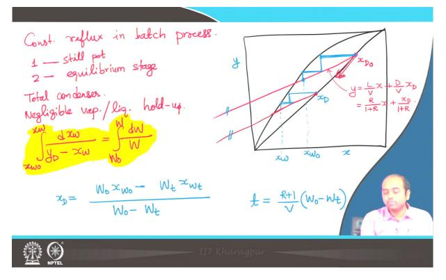
Let us try to work the graphical method once again. So, the only way to obtain constant distillate composition is by altering the reflux ratio. This is also true for continuous systems. The only way to obtain constant distillate composition is by altering the reflux ratio. How? So, let us say this is our y D. So, this is y versus x curve.
