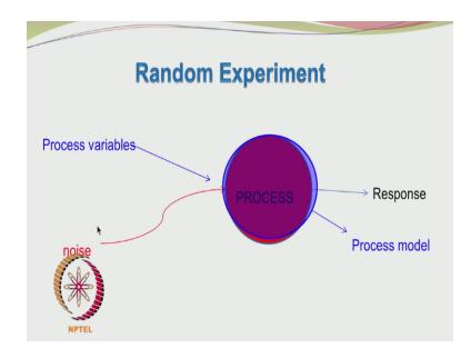
So this diagram shows the ideal process and the actual process. The ideal process which is one given by the model is shown by the blue diagram and here you have the process variables which are influencing the process. They are the inputs to the process model. You also have the unwelcome inevitable noise affecting the process and so you can even say that because of the effect of the noise which has not been accounted for in your model.
