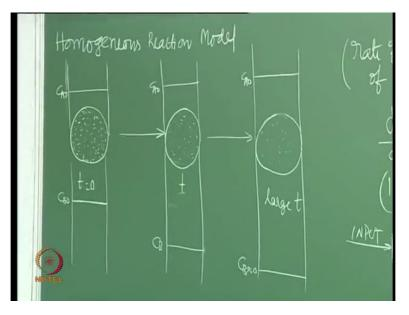
So we have a particle porous particle something like this then we have reactant B here reactant B and after sometime we have the same size particle we are talking about constant size but now this concentration will reduce then after sometime same particle the concentration is almost nil concentration of B I mean only product you will have so with time this is time t equal to 0, sometime t, large t good.
